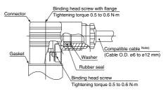
Note) For an outside cable O.D. ø9 to ø12 mm, remove the internal parts of the rubber seal before using.
