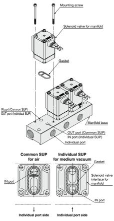
\* Mounting orientation exists when mounting valves onto manifold base. Mount it as shown above.
