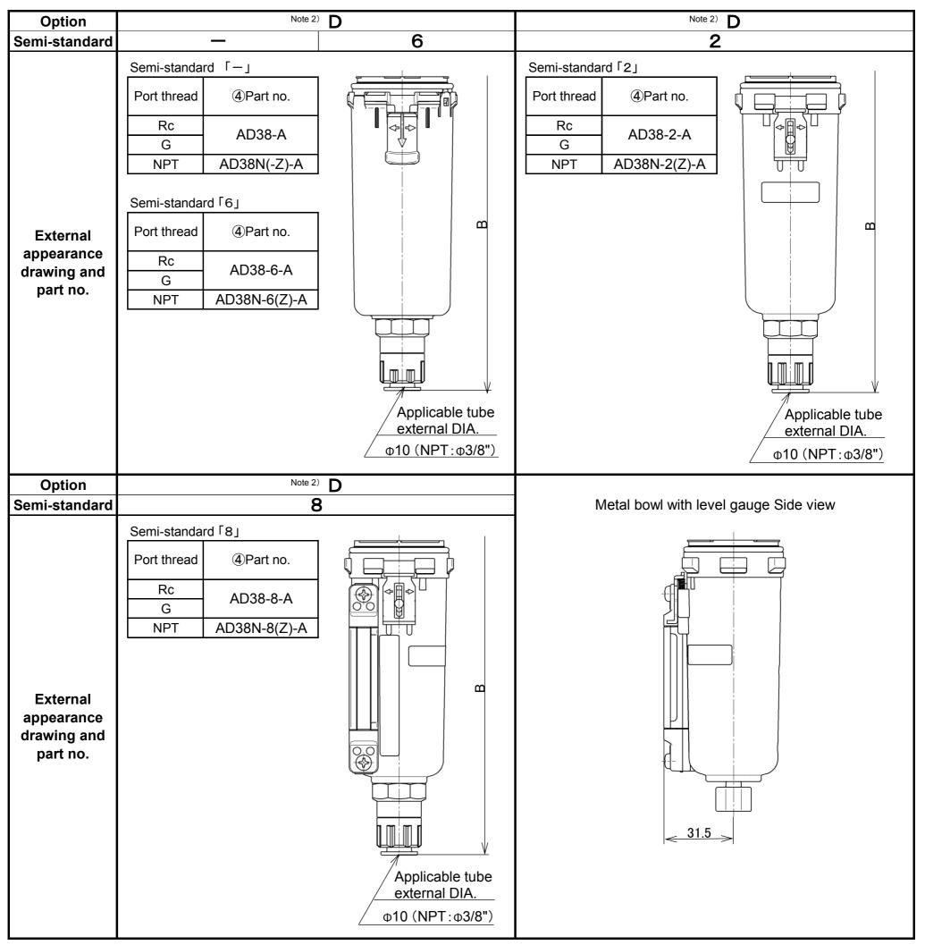
Note 1) B in the table shows the distance from inlet piping centreline to drain port. Refer to "12. DIMENTIONS" (P24). Note 2) Min. operating pressure is 0.15MPa for N.C. type and 0.1MPa for N.O. type.
