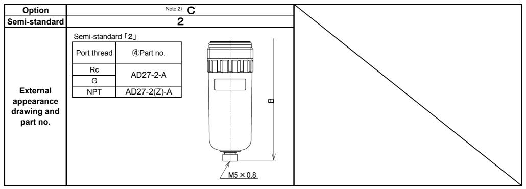
Note 1) B in the table shows the distance from inlet piping centreline to drain port. Refer to "12. DIMENTIONS" (P24).
