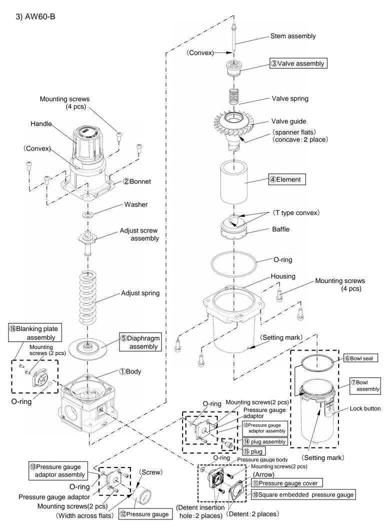
Note) If you want to install <code>(III)</code>Square embedded pressure gauge or <code>(III)</code>Pressure gauge adaptor assembly or <code>(III)</code>Plug assembly instead of <code>(III)</code>Blanking plate assembly, please contact SMC.
