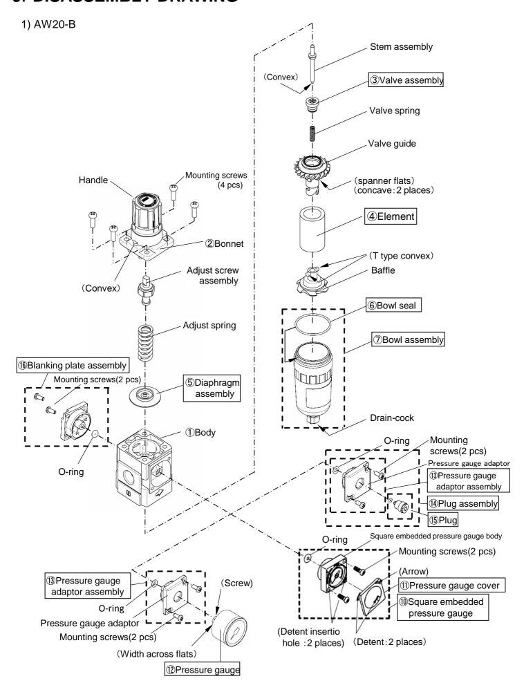
Note) If you want to install <code>(III)</code>Square embedded pressure gauge or <code>(II)</code>Pressure gauge adaptor assembly or <code>(II)</code>Plug assembly instead of <code>(II)</code>Blanking plate assembly, please contact SMC.
