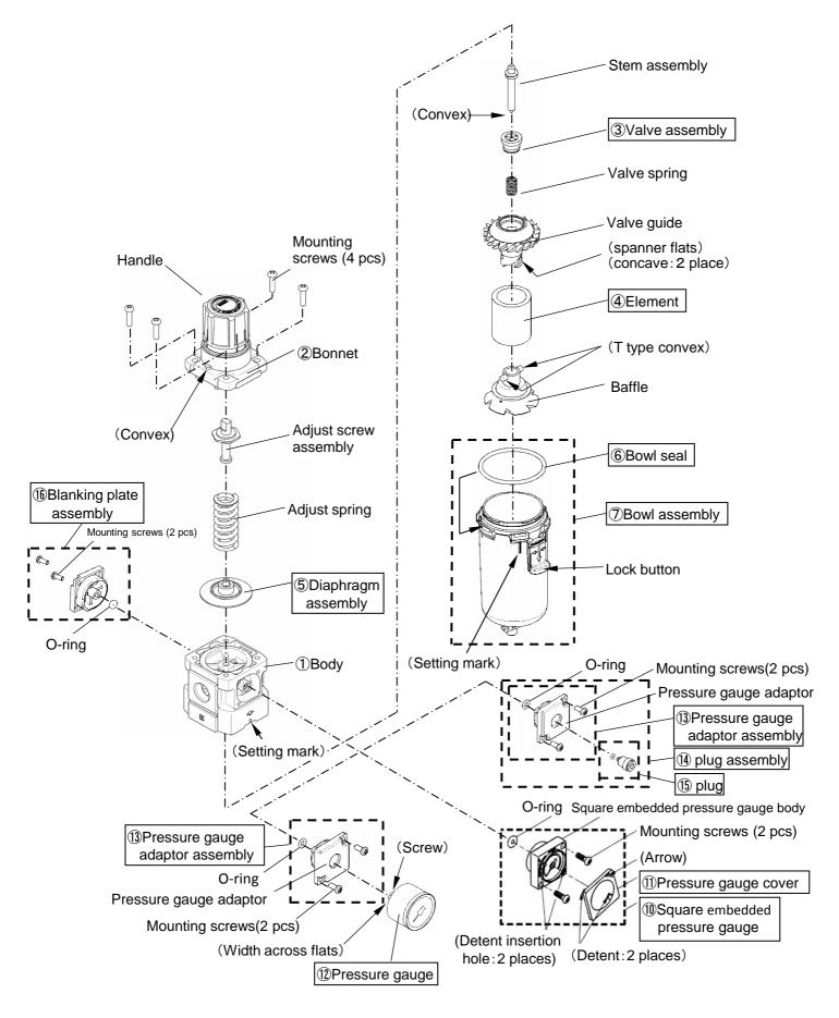
Note) If you want to install (1) Square embedded pressure gauge or (1) Pressure gauge adaptor assembly or (1) Plug assembly instead of (6) Blanking plate assembly, please contact SMC.
