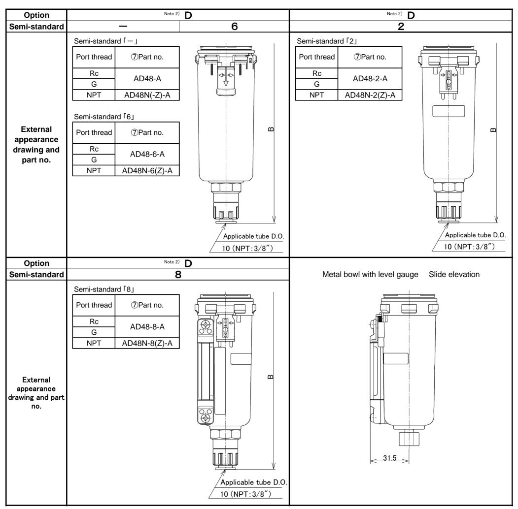
Note 1) B in the table shows the distance from inlet piping centreline to drain port. Refer to "10. DIMENTIONS" (P29).
