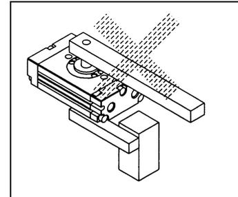
Inertia force generated by the load is directly applied to the axis if the external stopper on the opposite side of the load.
