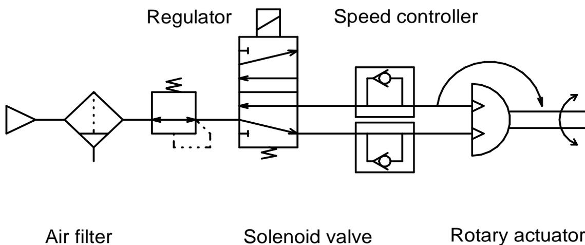
Fig.2 Basic circuit
