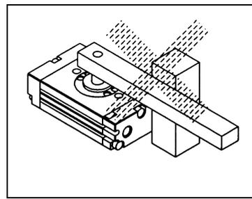
External stopper acts as fulcrum. Load inertia force is applied to the shaft as bending moment
