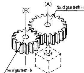
1. Calculate moment of inertia  $I_B$  around axis (B).
