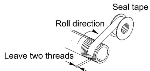
Fig.8 Applying seal tape
