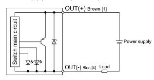
\*: The number marked on each lead wire color shows the pin number of pre-wired connector.
