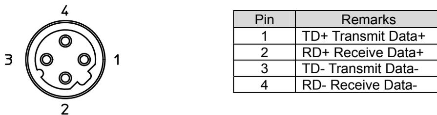
Fig. 6-5 Pin allocation of PROFINET connectors
