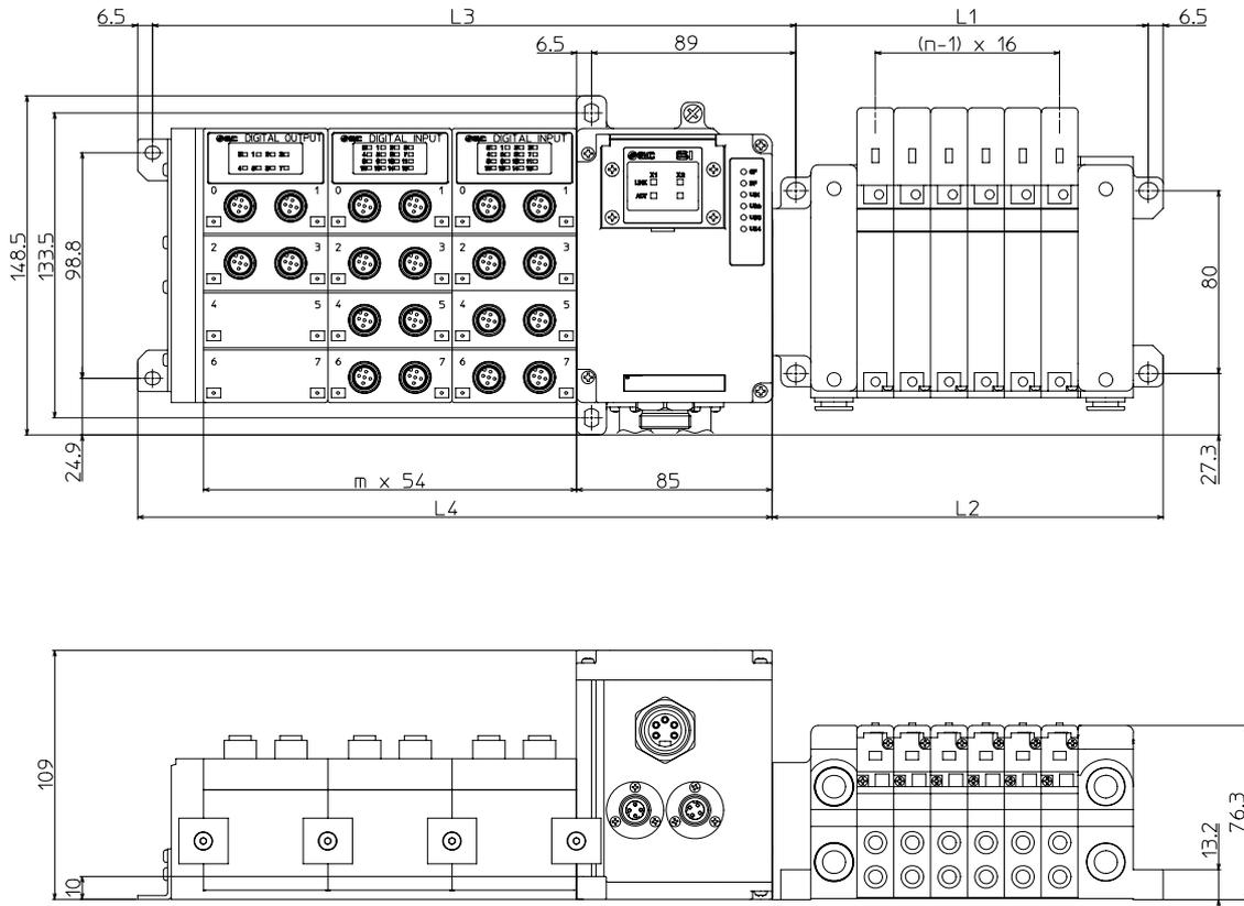
Fig. 14-2 Dimensions of the VQC2000 manifold
