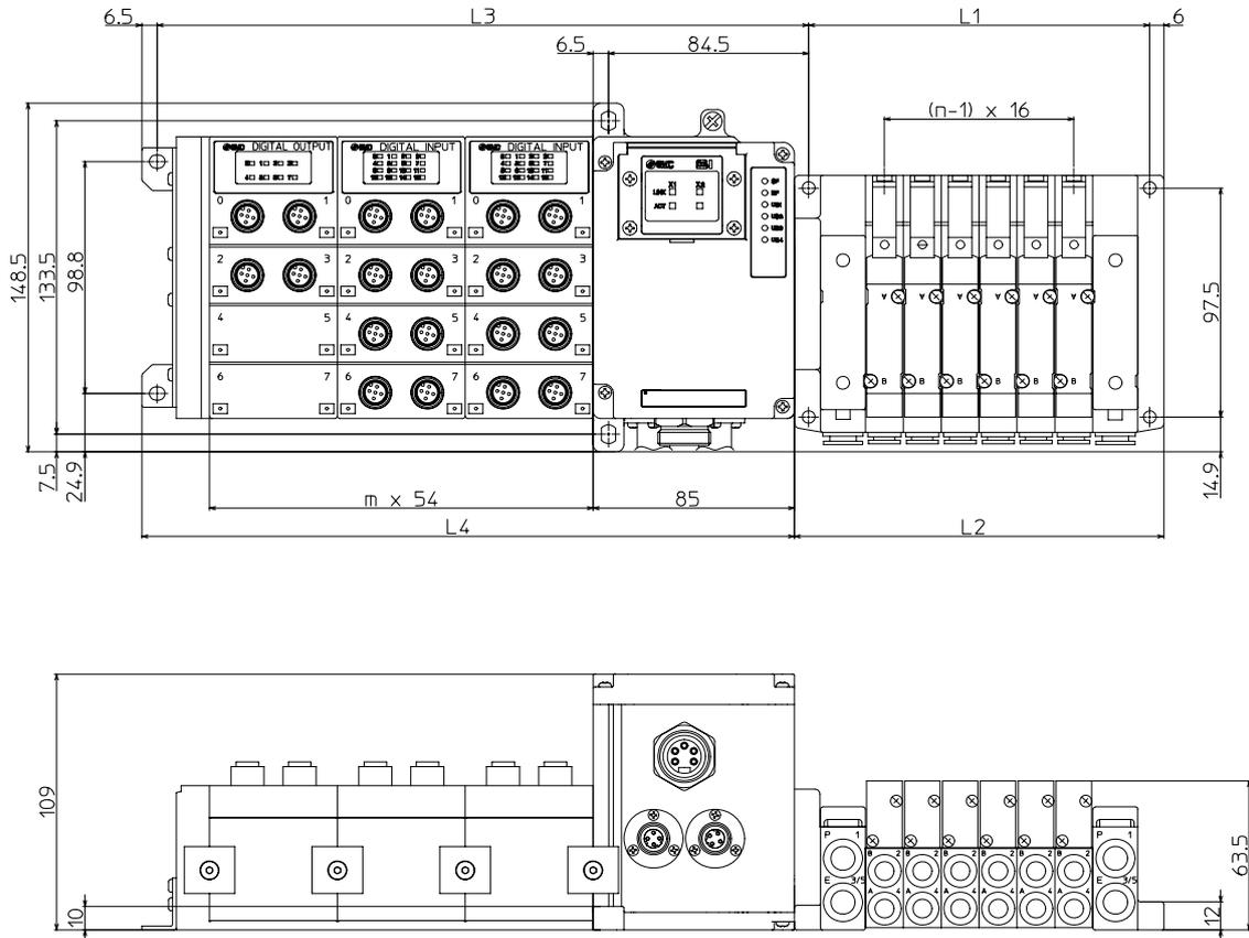
Fig. 14-5 Dimensions of the SV2000 manifold
