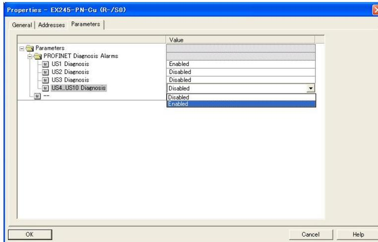
Fig. 7-10 System parameters of the EX245-SPR1-X171
