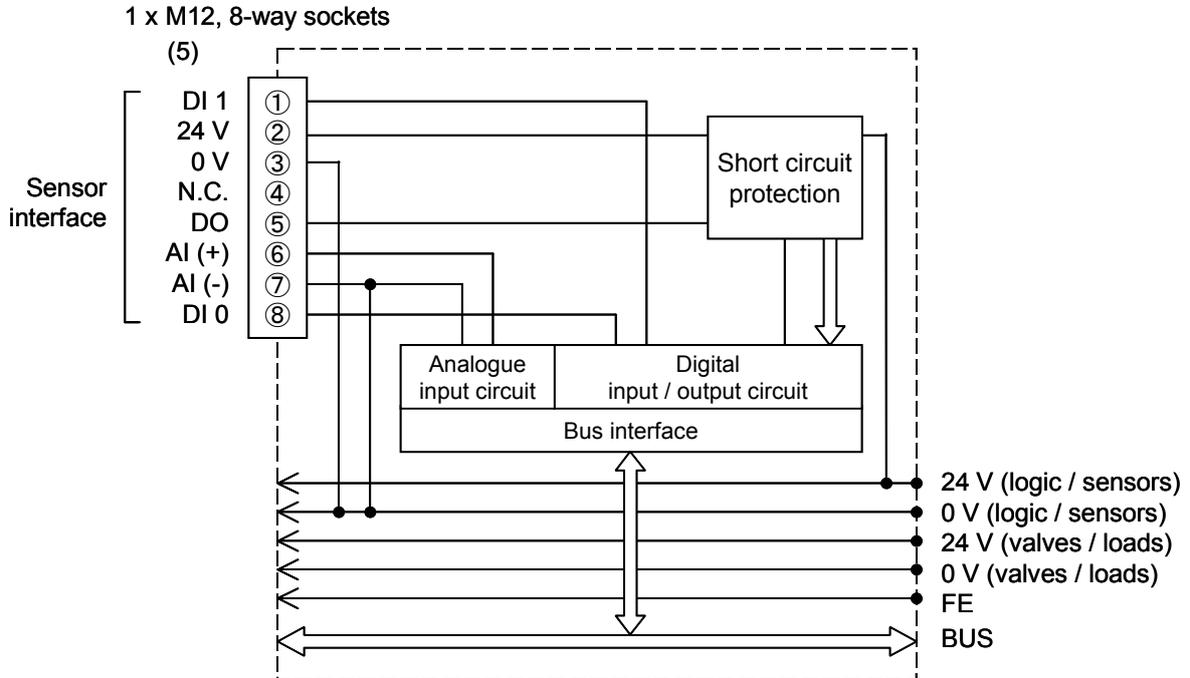
Fig. 13-3 Block diagram of the EX245-AX2-X38
