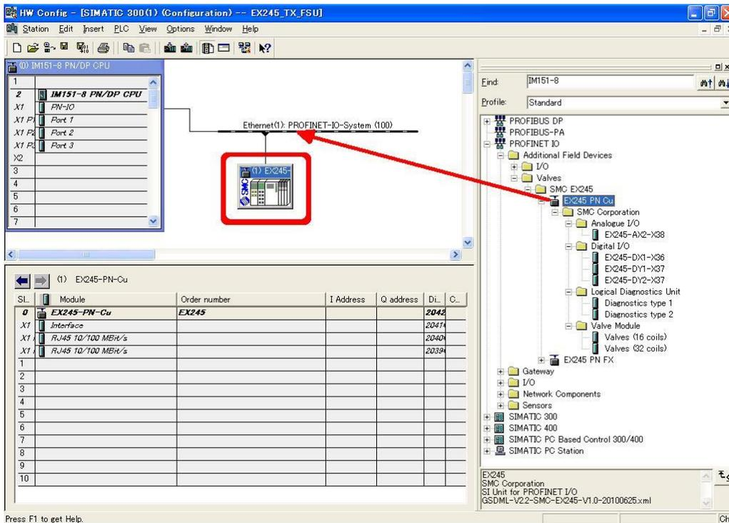
Fig. 7-7 Add EX245 onto a PROFINET network
