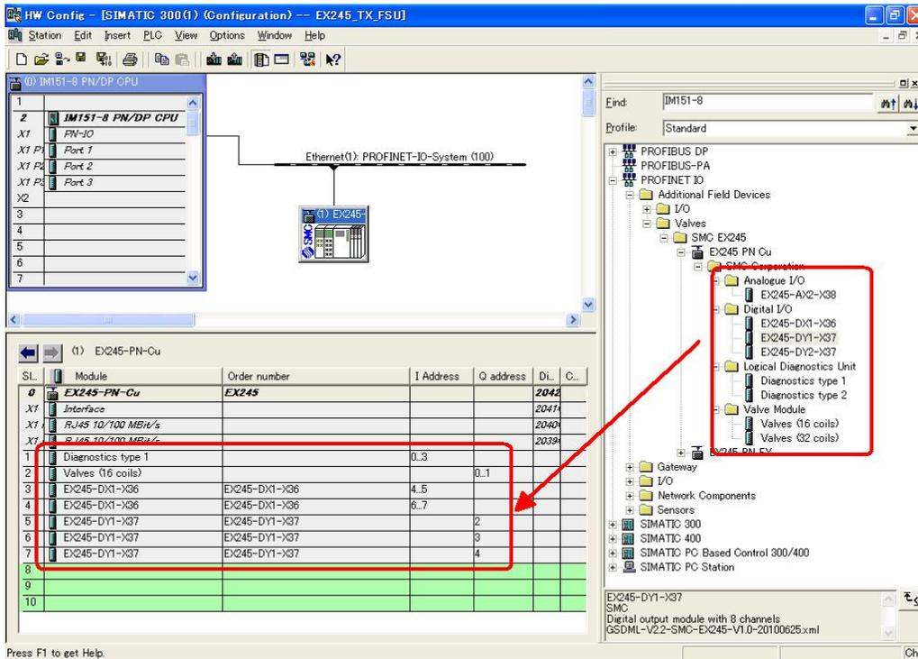
Fig. 7-9 Configure EX245 valve manifold
