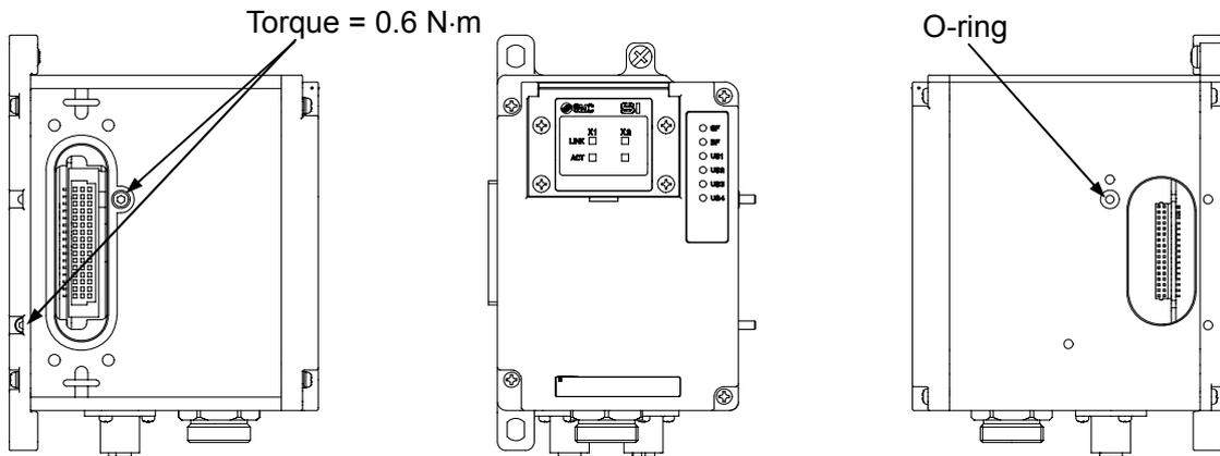
Fig. 6-2 Valve manifold connection
