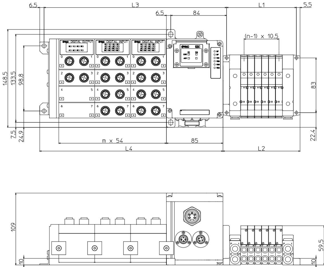
Fig. 14-4 Dimensions of the SV1000 manifold
