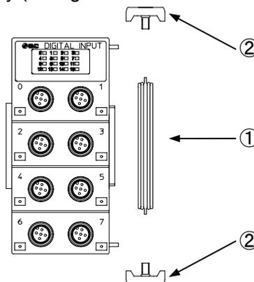
Fig. 6-3 Module connection
