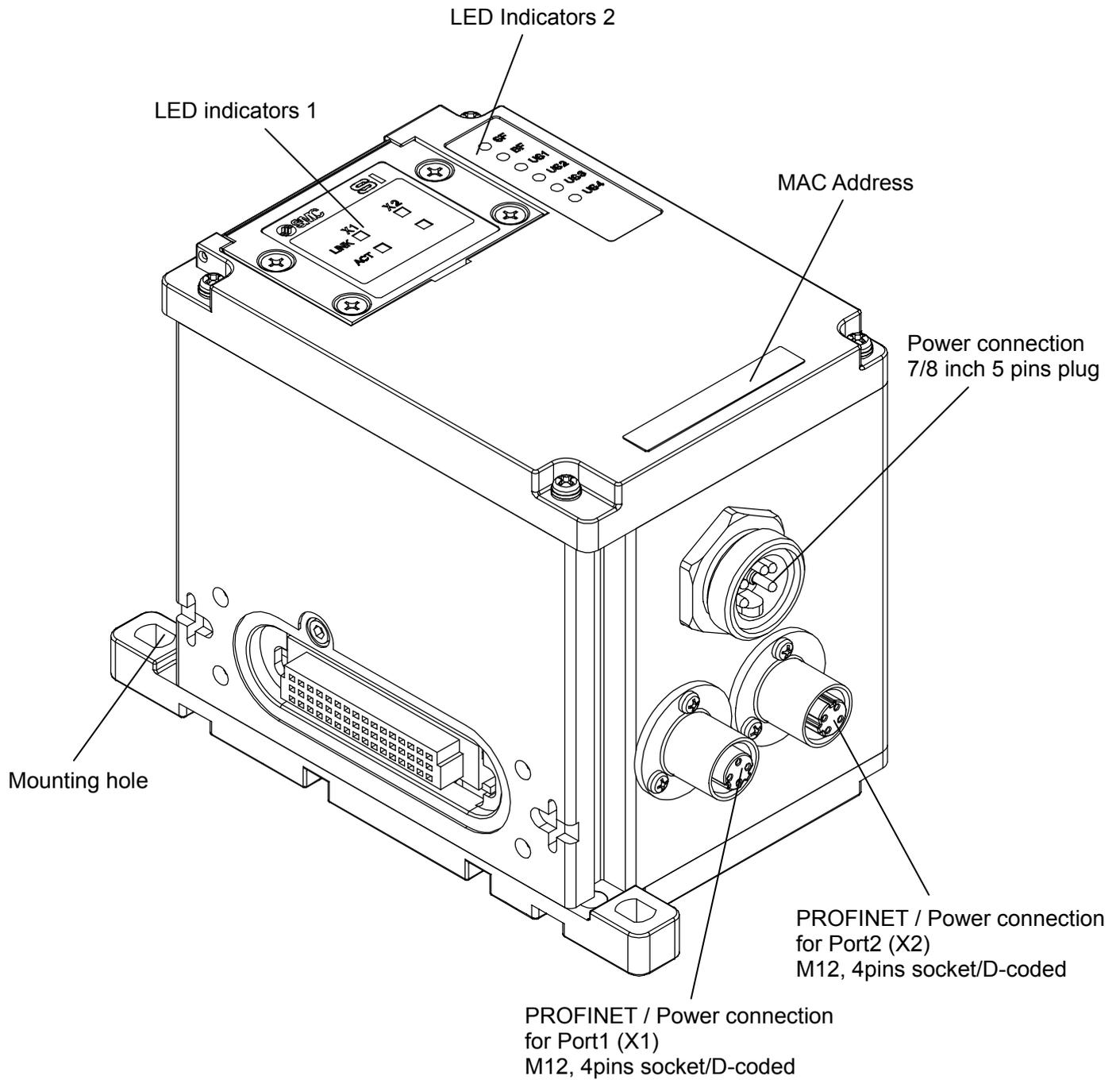
Fig. 9-1 Allocation of parts on the EX245-SPR1-X171
