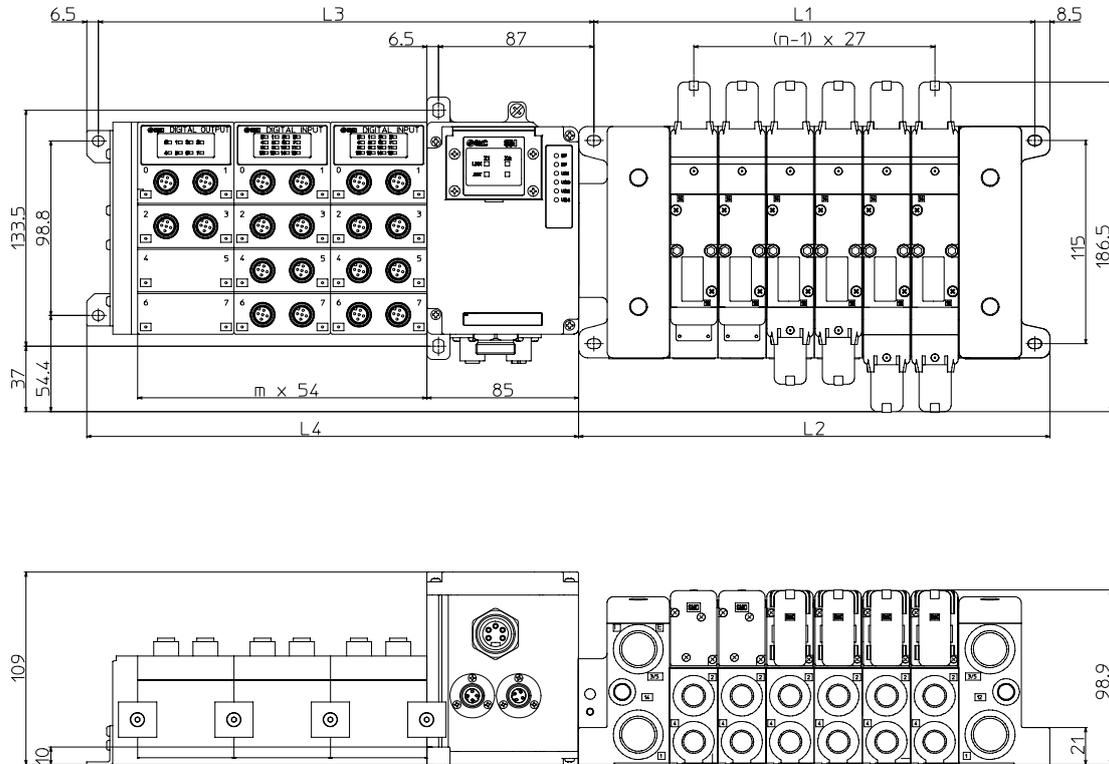
Fig. Fig. 14-8-Dimensions of the VSR8-4 / VSS8-4 manifold
