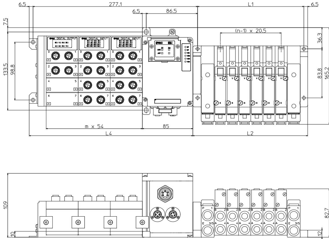
Fig. 14-6 Dimensions of the SV3000 manifold
