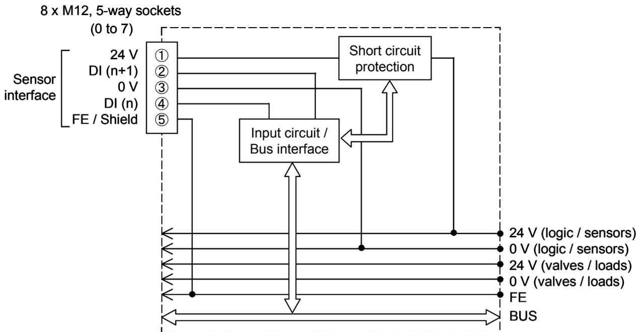
Fig. 10-3 Block diagram of the EX245-DX1-X36
