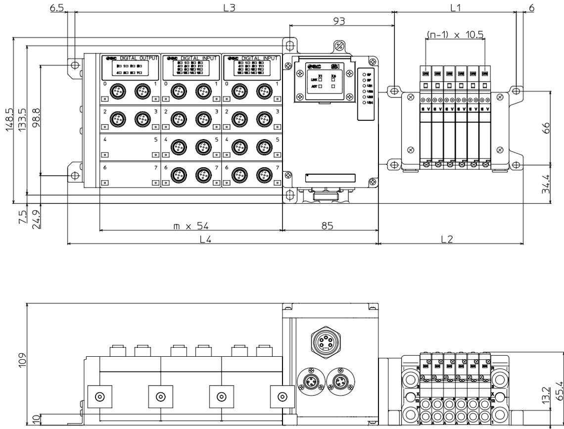
Fig. 14-1 Dimensions of the VQC1000 manifold
