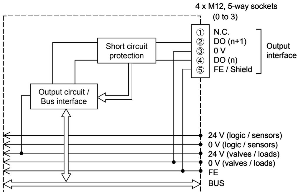
Fig. 11-3 Block diagram of the EX245-DY1-X37
