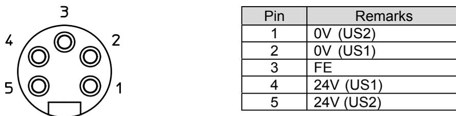
Fig. 6-4 Pin allocation of Power connector
