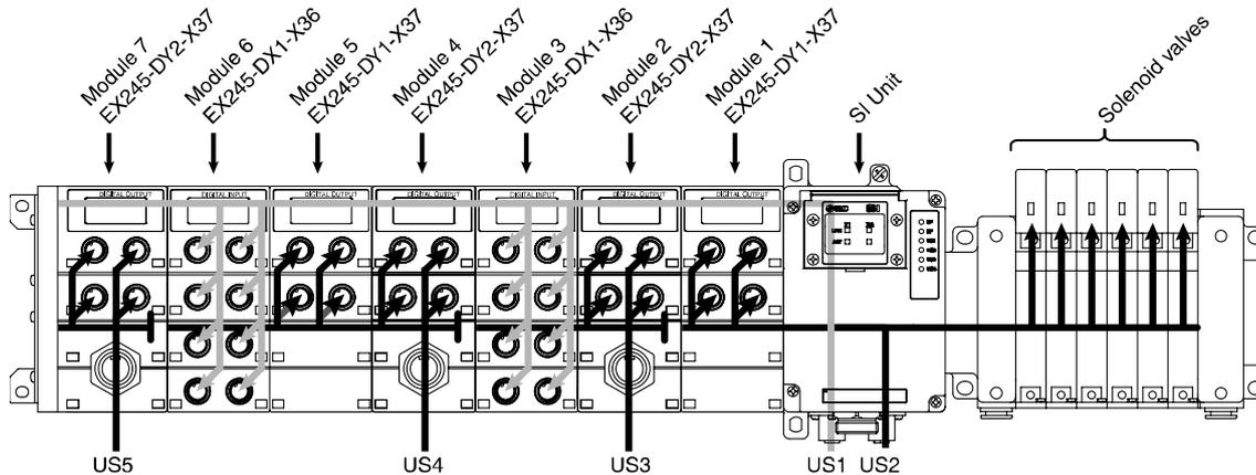
Fig. 4-1 Diagram of power supply concept (example)
