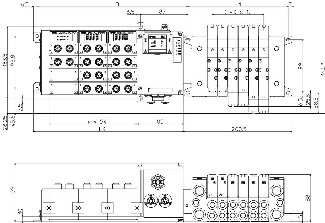
Fig. 14-7 Dimensions of the VSS8-2 / VSR8-2 manifold
