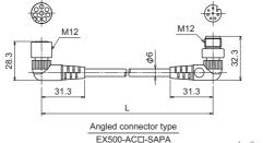
Minimum acceptable cable bending radius: 40 mm (fixed)
