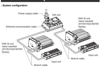
The EX500 range of units can be connected to open fieldbus (EtherNet/IP™) to realize the reduction of input or output device wiring and the distributed control system One branch of manifold valves/input unit can be connected to 32 outputs/32 inputs. Up to 4 branches can be connected (total 128 outputs/128 inputs)
