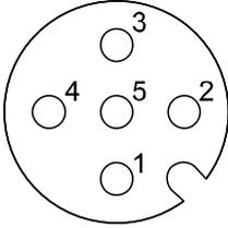
PWR: M12 5-pin plug, A-coded (SPEEDCON)
