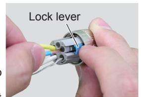
For CC-Link and DeviceNet™, insert the shield \*1 into terminal No.1 (grey).
