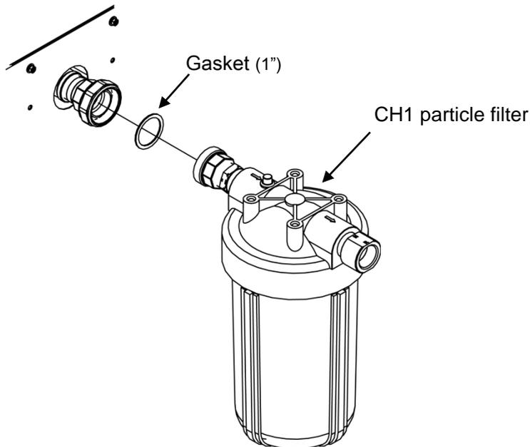
Fig. 3-15 CH1 side Installation of particle filter
