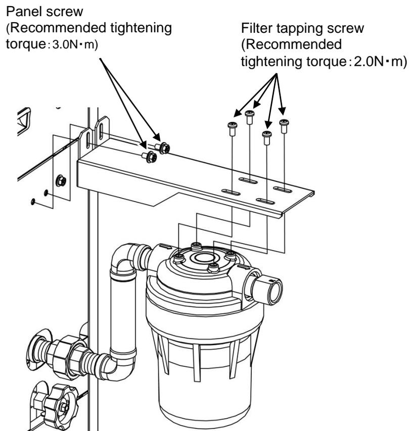
Fig. 3-19 CH2 side Installation of filter bracket.
