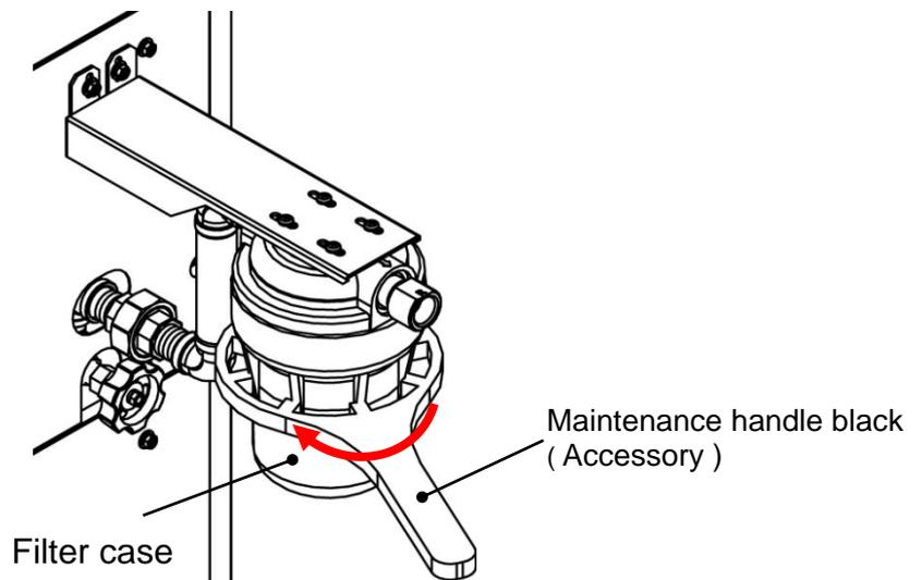
Fig. 3-21 CH2 particle filter case removal
