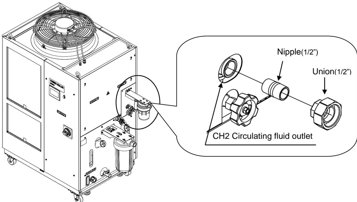
Fig. 3-17 CH2 side Tightening of piping
