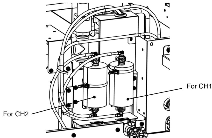
Fig. 7-5 Temporary pipe installation for DI filter(For option D1)
