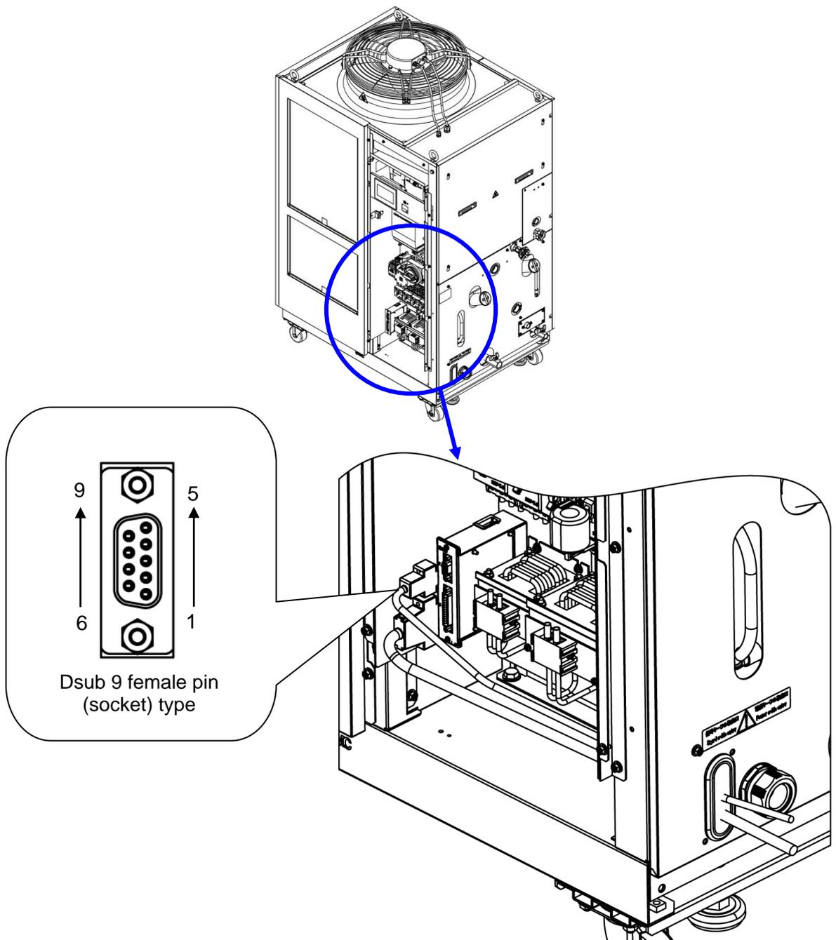
Fig. 3-12 RS-485 communication wiring
