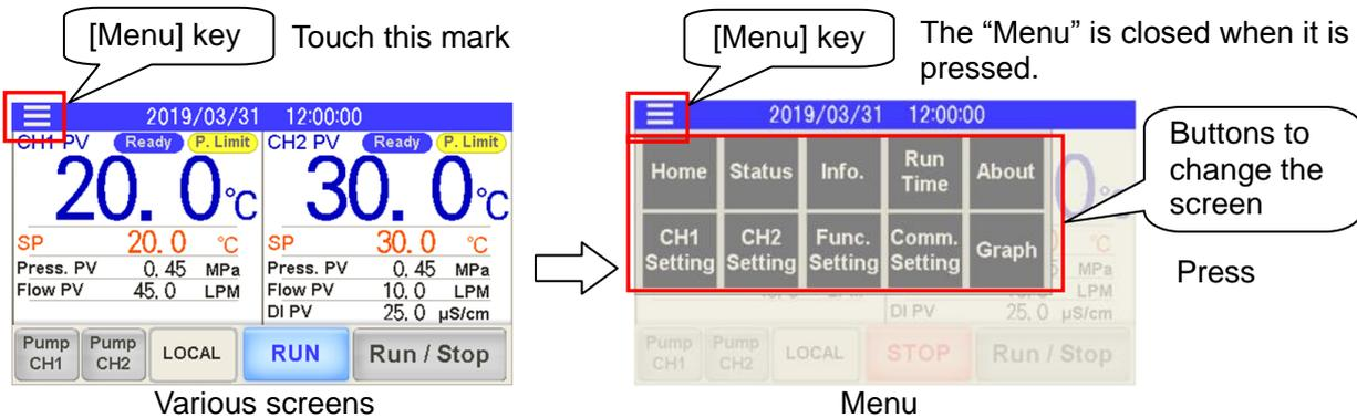
3. Press a button for example to carry out "Run/Stop," "Selection of function" or "Change the screen.
