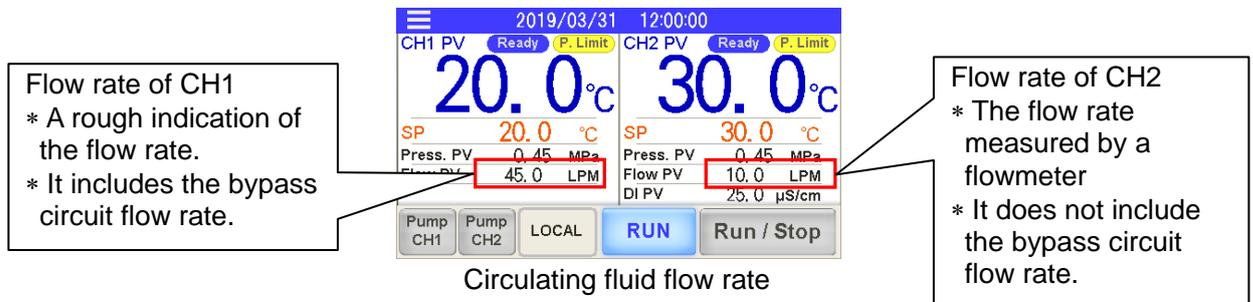
•Circulating fluid flow rate [DI PV]
