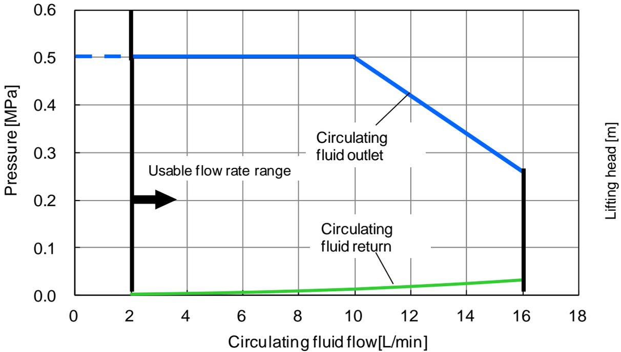
Fig. 8-12 Pump capacity(HRL100/200/300-A\*-40 CH2)
