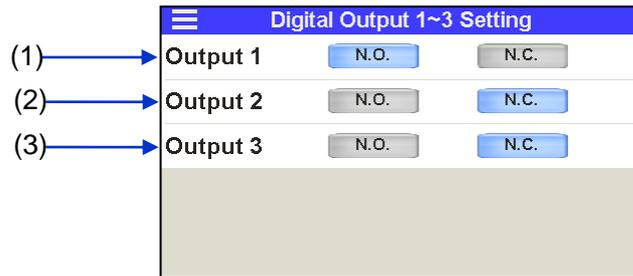
Setting of contact output signal 1 to 3
