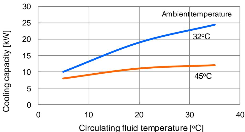
\*This is the cooling capacity of the CH1 side when 1 kW heat load is applied to the CH2 side.
