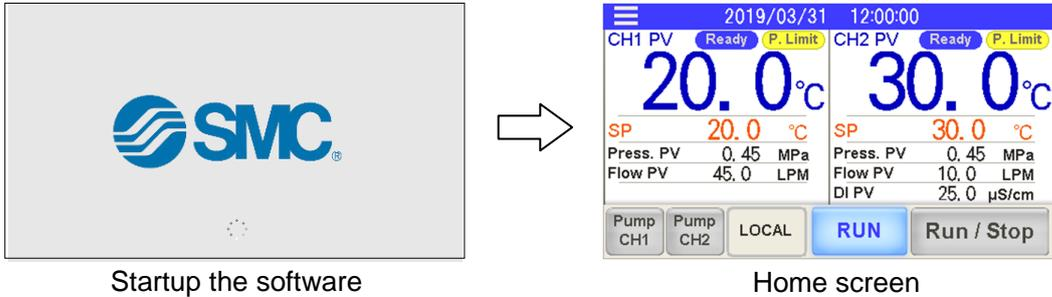
2. Settings and screen display can be reviewed after the home screen changes to the respective screen. The menu is displayed when [Menu key] (three horizontal lines) located upper left on the screen is touched. Go to the respective screen from the menu to check the settings and screen display content.
