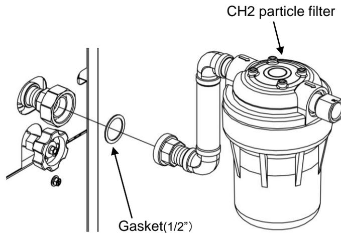
Fig. 3-18 CH2 side Installation of particle filter
