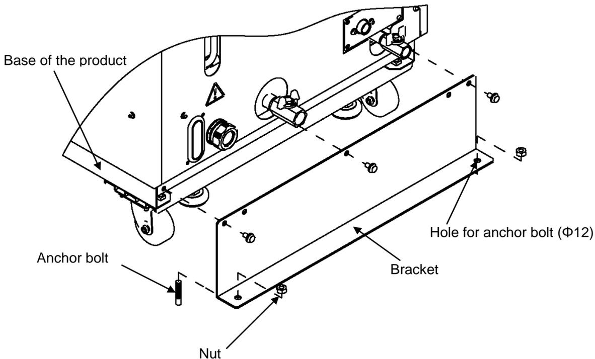
Fig. 3-4 Installation procedures
