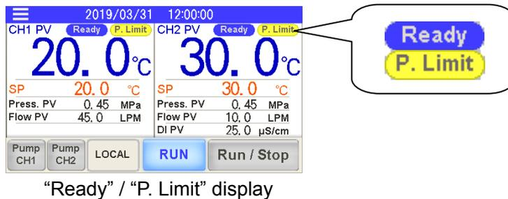
• Current circulating fluid temperature [PV]
