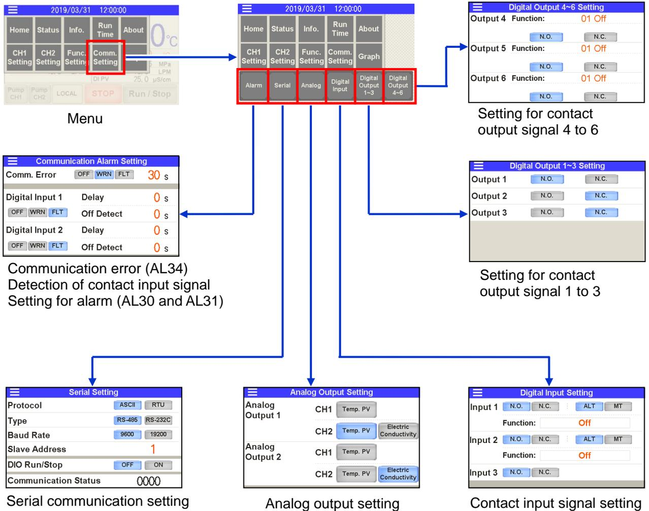
• Setting for communication error (AL34)/contact input signal detection (AL30 and AL31)
