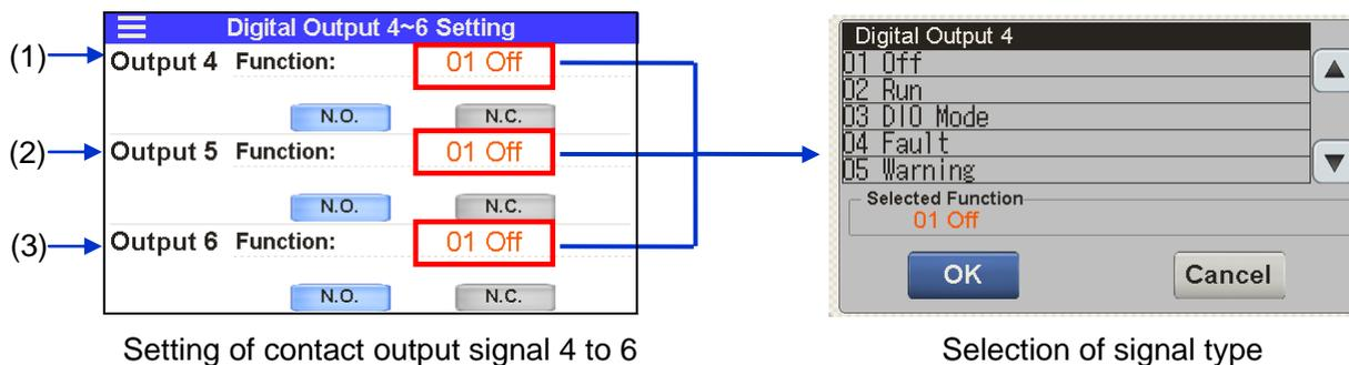
Setting of contact output signal 4 to 6
