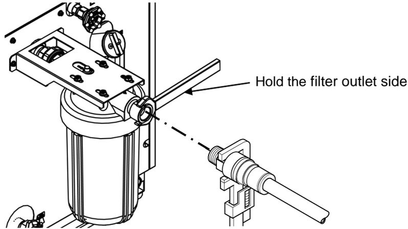
Fig. 3-22 Hold the filter outlet side
