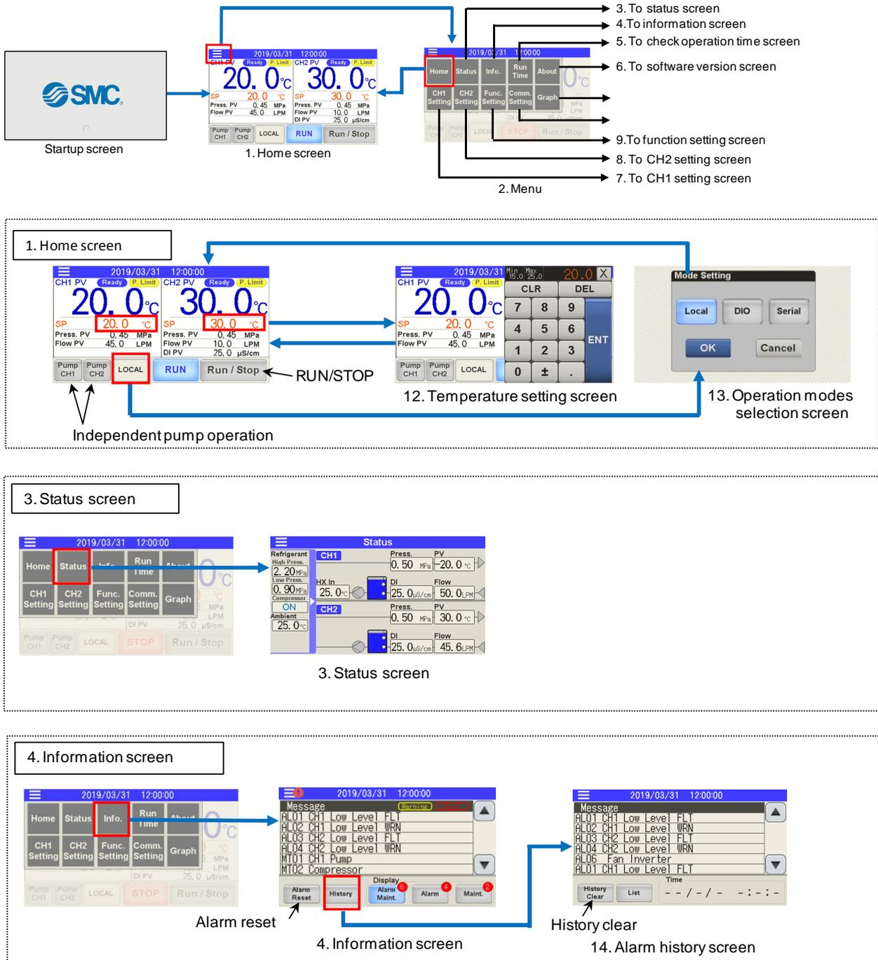
Fig.5-2 Flow chart of operation screen (1/3)
