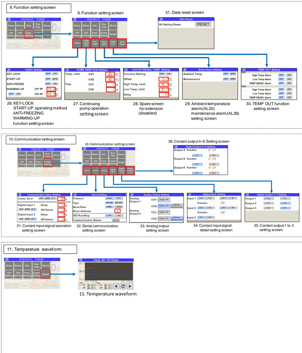
Fig. 5-4 Flow chart of operation screen (3/3)
