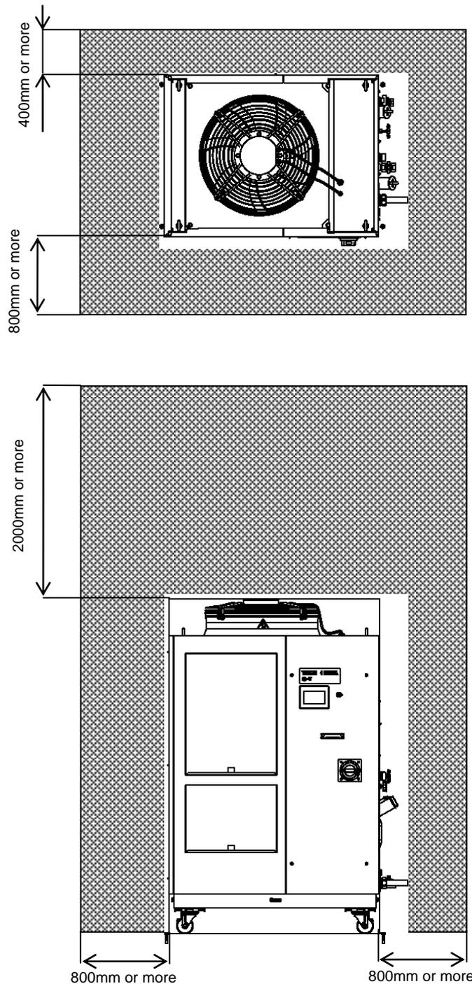
Fig. 3-3 Installation space (This drawing shows "HRL200-A-20".)
