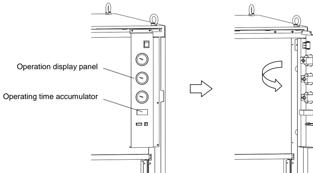
3. Disengage the hooks on the top and bottom of the case with a tool.
