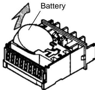
6. Before inserting the battery, wipe off its surface for cleaning.
