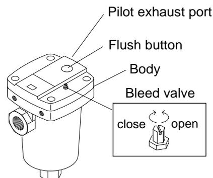
[Disassembly and cleaning of auto drain]
