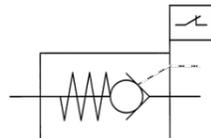
The intended use of this product is to stop the flow of pressurized air in one direction and to detect the safe state of the check valve for diagnostics in safety related circuits.
