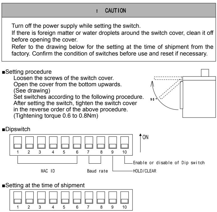
Node address: 0 Baud rate: 125kbps Hold/Clear: Clear Dip switch: enable
