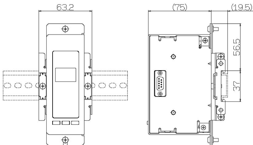
High voltage power supply module (IZTP40, IZTP41)
