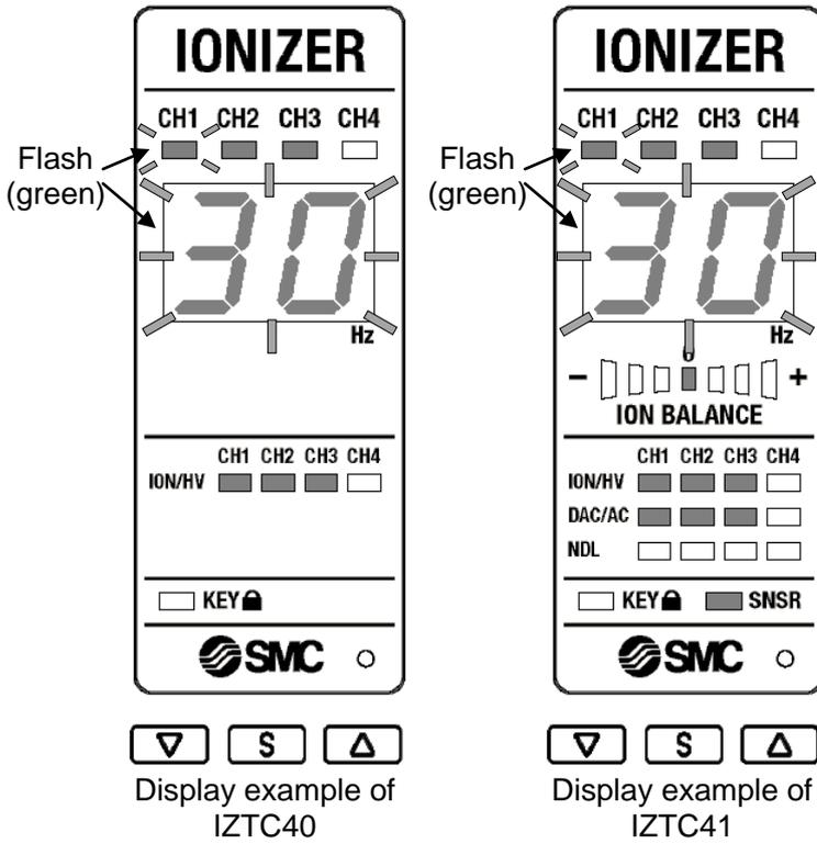
Example of frequency setting mode for CH1.
