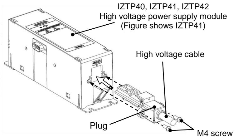
Tightening Torque: 0.49 to 0.53 Nm
