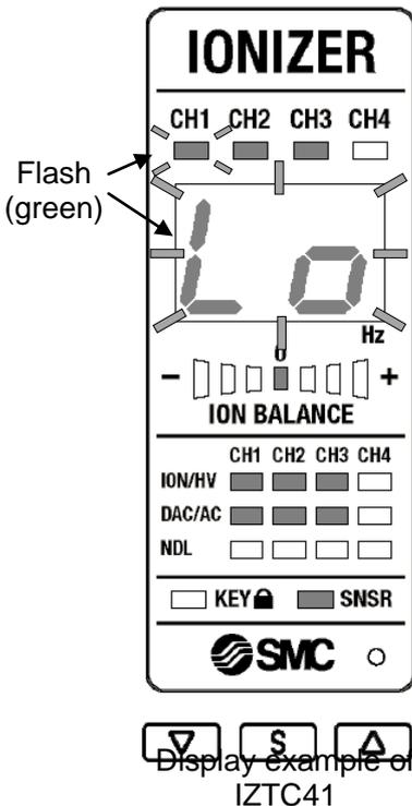
Example shows the emitter contamination detection level of CH1.
