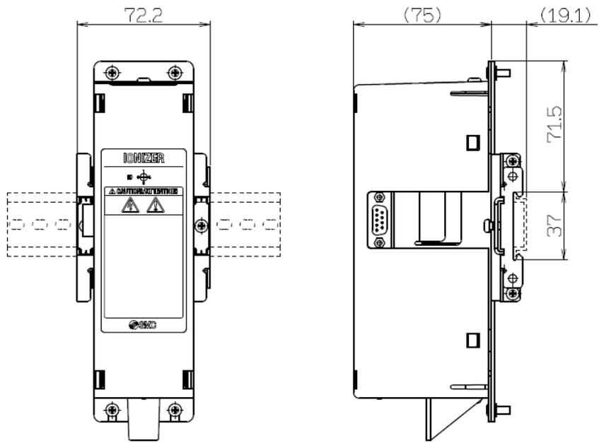
High voltage power supply module (IZTP42)
