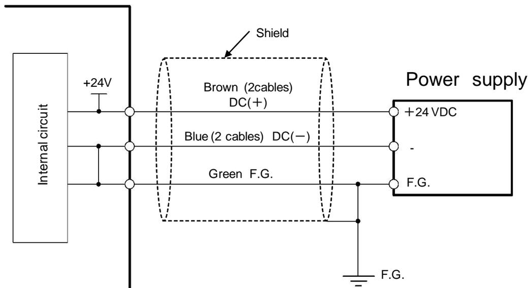
When the product is used in DC mode, make sure to ground the F.G. cable (green) and DC(-) cable (blue) of the input power supply **with a resistance of 100 ohms or less.** Without grounding the DC(-) cable, the ionizers and/or power supply may be damaged.
