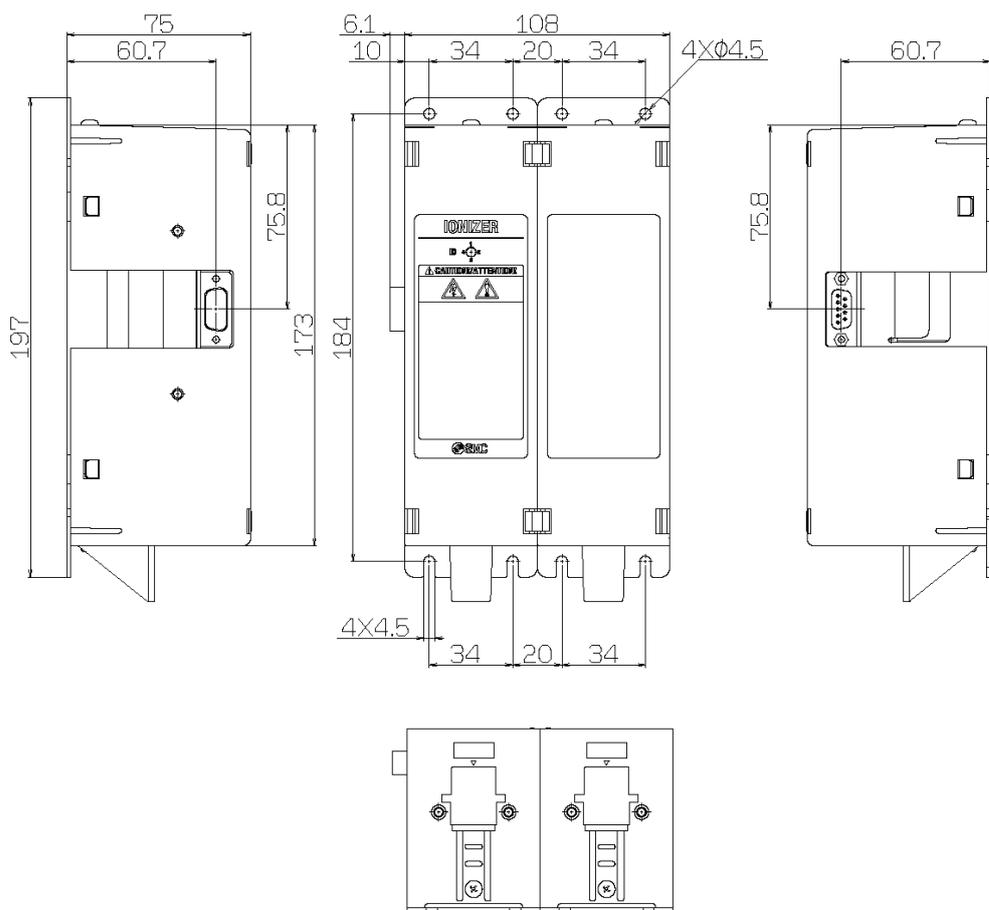
When DIN rail mounting bracket (IZT40-B3) is used
