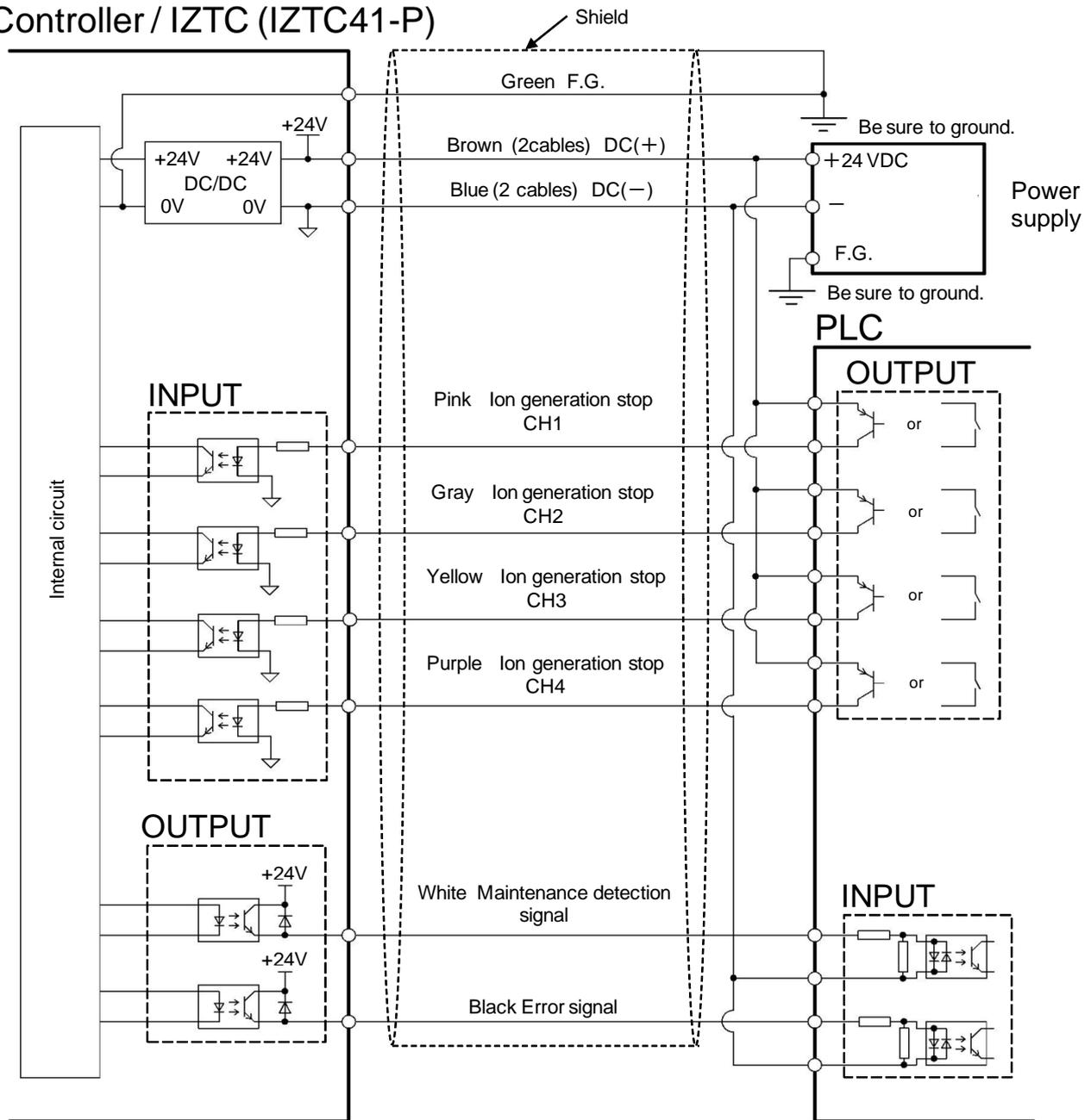
When an ionizer (IZT41) is used in DC mode, make sure to ground the F.G. cable (green) and DC(-) cable (blue) of the input power supply **with a resistance of 100 ohms or less**. Without grounding the DC(-) cable, the ionizers and/or power supply may be damaged.
