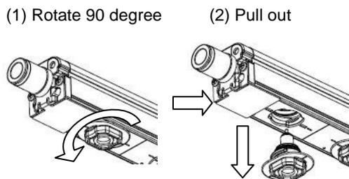
Removal procedure of emitter cartridge
