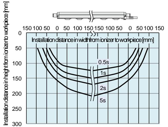
2) With High speed static neutralization cartridge, Supply pressure: 0.3 MPa
