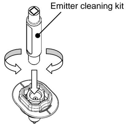
d. When the emitter cartridges are removed for cleaning, remount them to the ionizer according to the "Mounting procedure of emitter cartridge" shown below. Make sure that the cartridges are securely mounted. If not, the cartridges may become dislodged when compressed air is supplied to the ionizer.
