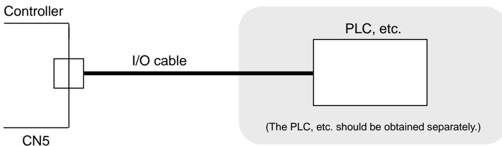
Please refer to "6.4 Parallel I/O Wiring Example" for how to wire the CN5 connector.
