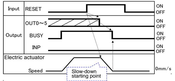
If the electric actuator is within the "In position" range, INP will be turned ON.
