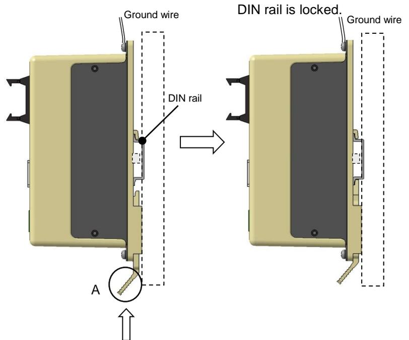
Hook the controller on the DIN rail and press the lever of section A in the arrow direction to lock it.
