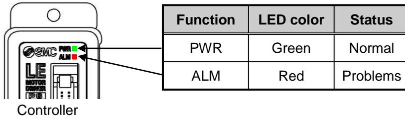
If the LED [PWR] lights in green, the controller is in the normal condition.
