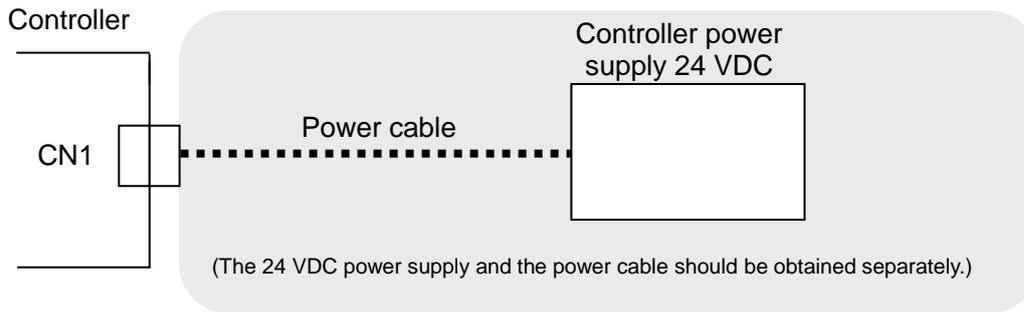
Please refer to “5. CN1: Power supply plug” for how to wire the CN1 connector.
