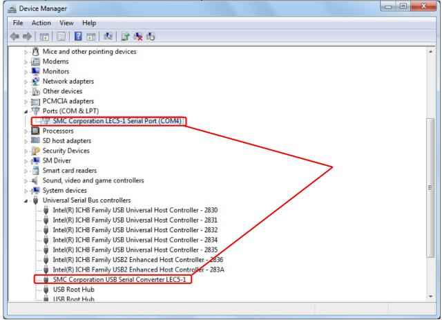
The communication port number is needed when starting this software.
