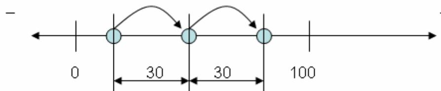
In this example, the moving distance is 30 mm. The table moves 30 mm each from the current position. It does not mean that the target position is 30 mm away from the origin position.
