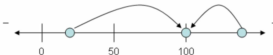
In this example, the target position is 100 mm as absolute positioning. The table moves to the position of 100 mm regardless wherever the table is.
