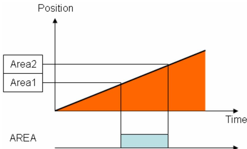
The AREA output is a signal to be output when the position enters the specified range. The AREA 1 and AREA 2 in the setting items define this output range.
