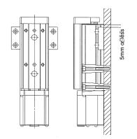
**20.** The product should be mounted as shown below in the figures marked with the O. Unstable mounting of the product may cause operation failure, generation of abnormal noise or increase in the deflection etc.
