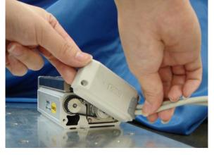
3. Loosen the bolts fixing the motor. Do not remove the bolt completely to avoid loosing them.
