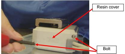
2. Displace the cover holding the cable. (If the cable is pulled forcefully, it will be disconnected)
