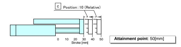
Condition 2) 30mm position  $\rightarrow$  **Step no.1**  $\rightarrow$  **Step no.1** (Move M: Relative)
