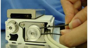
6. Set a new belt. Mount the motor pulley with belt tension force below.
