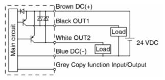
Max.80 mA Internal voltage drop 1.5 V max.
