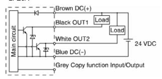
Max.28 V, 80 mA Internal voltage drop 1 V max.
