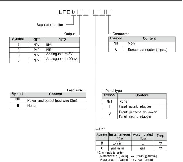
\*: For the remote sensor, select analogue output: 1 to 5 V type . Applicable sensor: LFE $\Box$ J $\Box$
