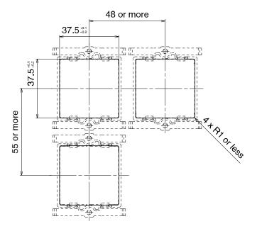
\*: The thickness of the panel is 0.5 to 0.8mm (with a waterproof seal: 0.5 to 6mm).
