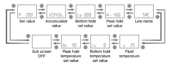
The set values of OUT2 and accumulated output cannot be displayed. (Example for 20 L/min type the above) \* Temperature peak, temperature bottom, and fluid temperature display are items which are not used for this product.
