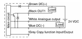
Max.28 V, 80 mA Internal voltage drop 1 V max. Analogue output 1 to 5 V Output impedance 1  $k\Omega$
