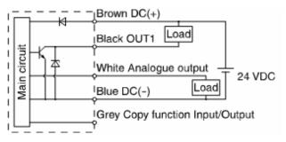
Max.28 V, 80 mA Internal voltage drop 1 V max. Analogue output 4 to 20mA Max. load impedance 600  $\Omega$
