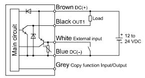
Maximum 28 V, 80 mA Internal voltage drop 1 V or less External input: Voltage free contact
