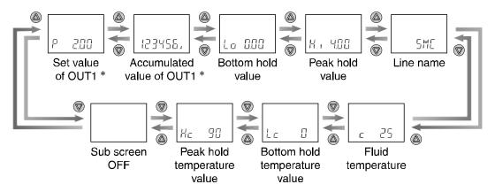
\*: The set values and accumulated output of OUT2 cannot be displayed.
