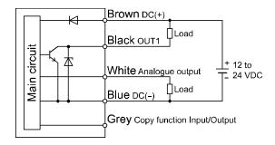
Maximum 28 V, 80 mA Internal voltage drop 1 V or less C: Analogue output 1 to 5 V
