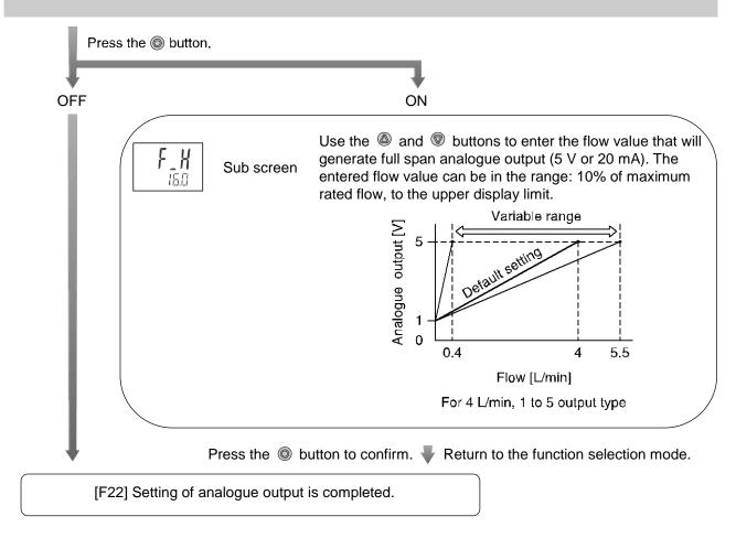
\*: The analogue output of the remote sensor is saturated at approx. 5.6 V, so use it with 110% or lower of maximum rated flow.
