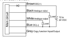
J: Analogue output 1 to 5 V Output impedance 1  $k\Omega$
