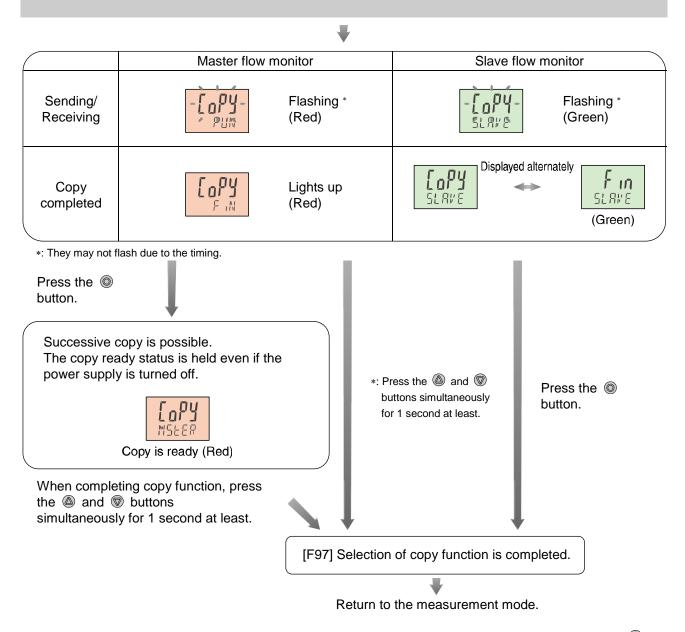
\*: It the copy to the slave flow monitor is not completed, it is detected as a copying function sending/receving error. Press the and buttons simultaneously for 1 second at least to return to the measurement mode. Then, check the wiring of the switch and retry copy function.
