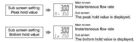
The maximum (peak) and minimum (bottom) flow from when the power is supplied to this moment is detected and updated.
