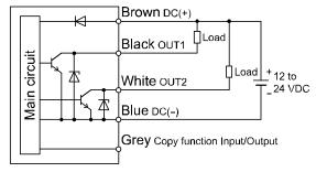
Maximum 28 V, 80 mA Internal voltage drop 1 V or less
