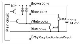
Maximum 80 mA Internal voltage drop 1.5 V or less
