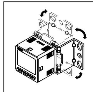
\*Bracket can be mounted on 4 sides.
