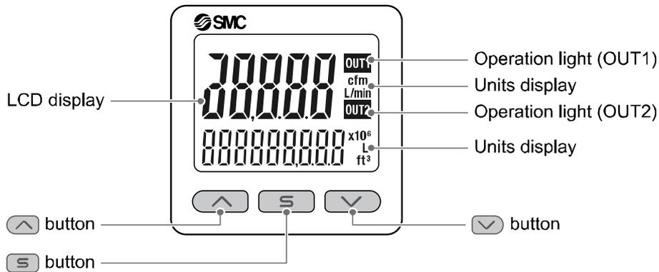
Operation light: Displays the switch operating condition.
