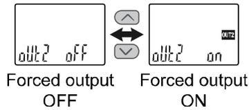
When switching of analogue output is selected for the setting of [F 5] FUNC terminal function
