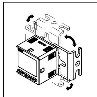
\*Bracket can be mounted on 4 sides.
