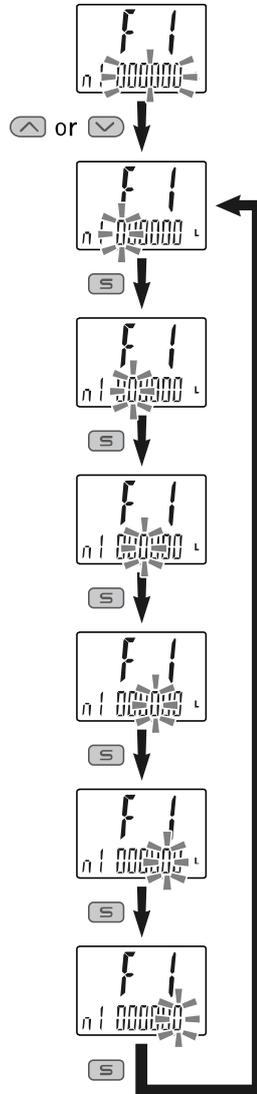
When the **S** button is pressed for 1 second or longer, the flashing will stop.
