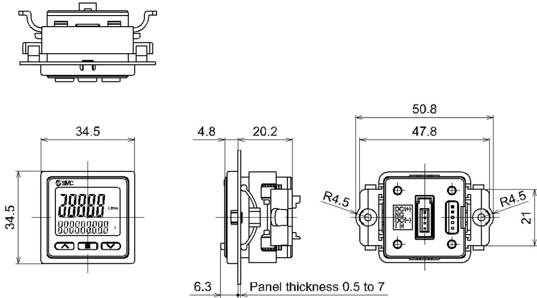
○Panel mount adapter + Front protective cover (Part No: ZS-46-D)
