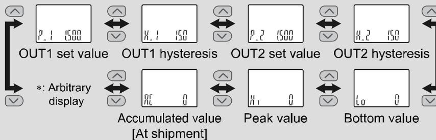
\*: One arbitrary display mode can be added to the sub display by setting the [F10] sub display setting. (The default setting does not include arbitrary display.)
