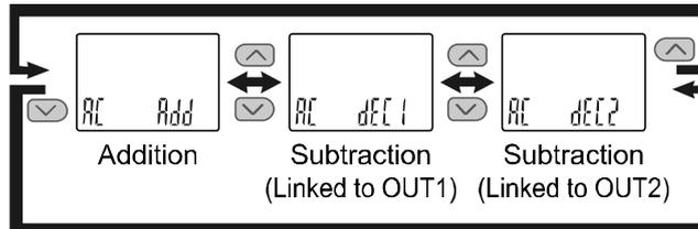
Press the button to set. Move on to accumulated value setting.
