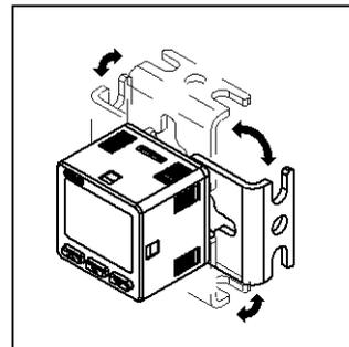
\*Bracket can be mounted on 4 sides.
