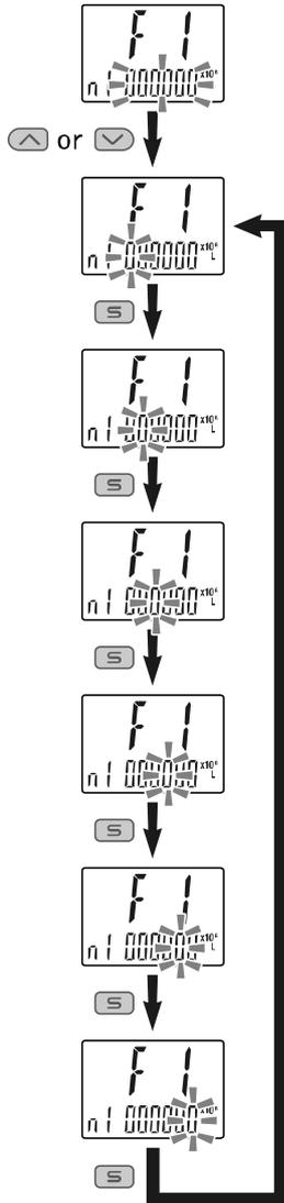
When the **S** button is pressed for 1 second or longer, [000000] will start flashing.
