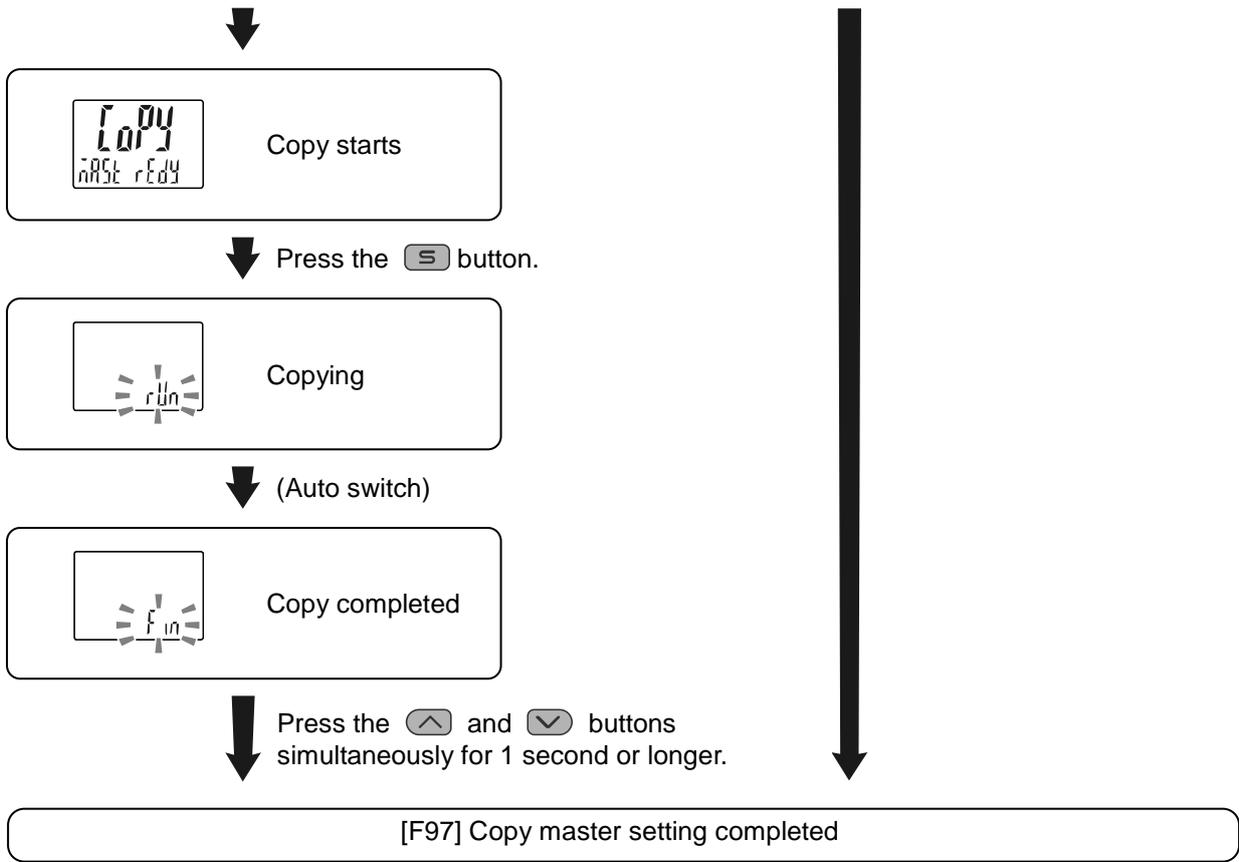
After selecting the copy master, all other connected monitors switch to slave mode.
