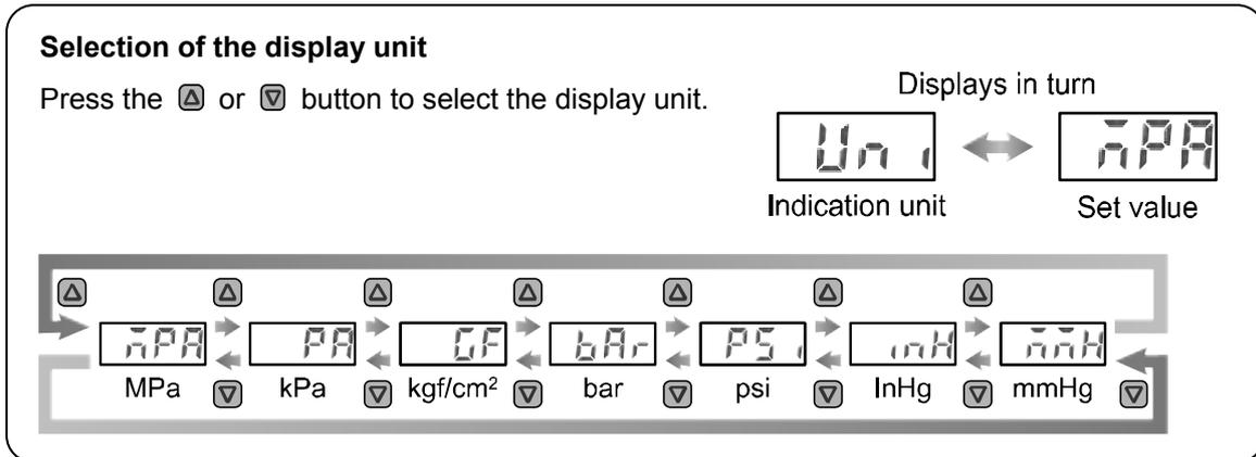
Press the  $\text{S}$  button to set.  $\downarrow$  Return to function selection mode.
