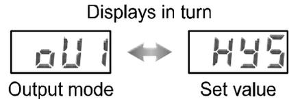
Press the **S** button to set. **↓** Move on to setting of reversed output.
