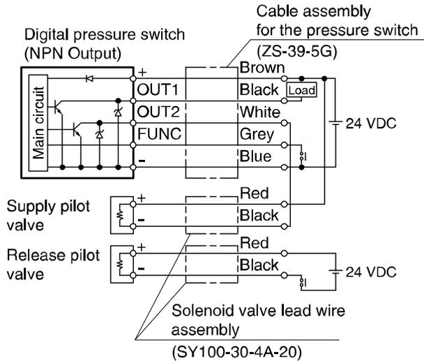
Integrated electrical entry for the pilot valves and the digital pressure switch
