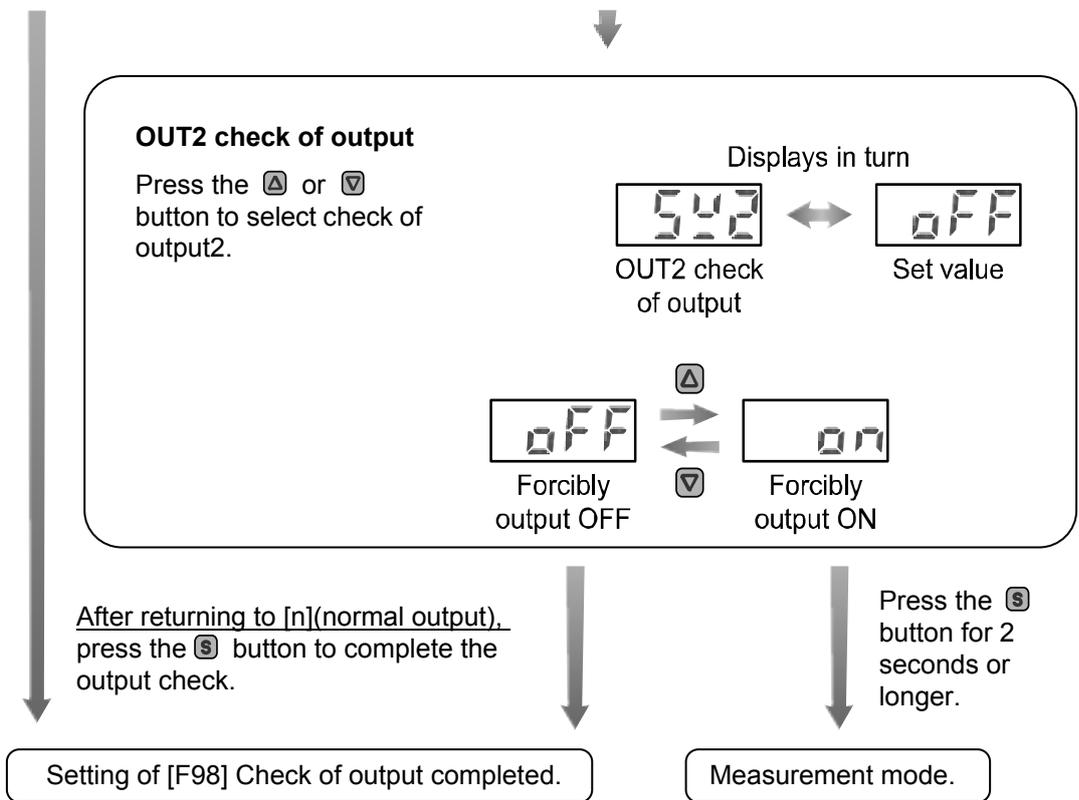
\*: Return to measurement mode from any point by pressing the S button for 2 seconds or longer.
