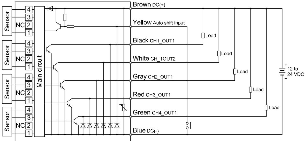
**PSE201-(M)** □: PNP open collector 5 outputs + Auto-shift 1 input
