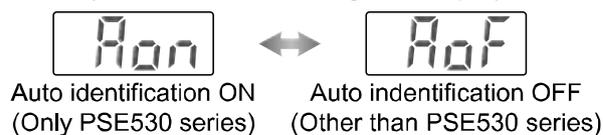
\*: Setting for the automatic identification function is ON when default setting.
