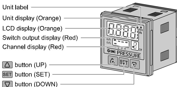
Switch output display (Red): Lit when OUT1 (CH1 to CH4) and/or OUT2 (only CH1) is ON.
