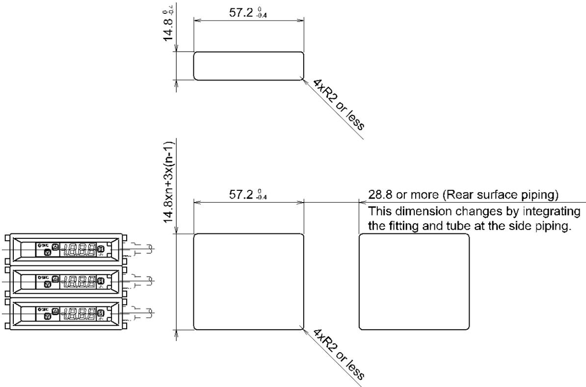
○DIN rail mounted side piping
