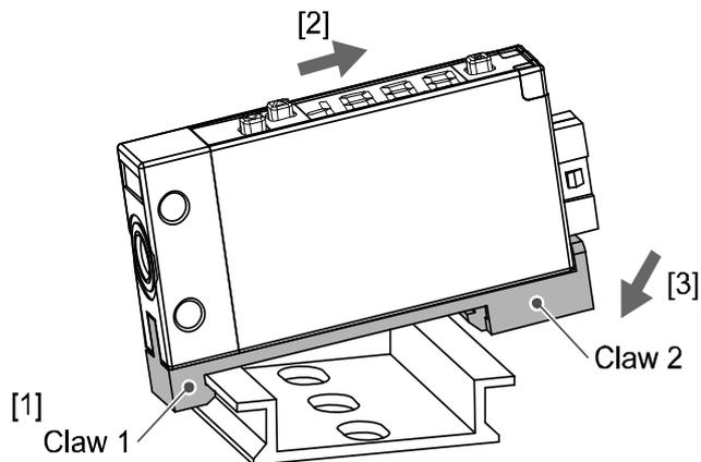
Engage claw 1 of the adapter on to the DIN rail as shown [1], apply force in direction [2], then press downward [3] until claw 2 clicks on to the DIN rail.
