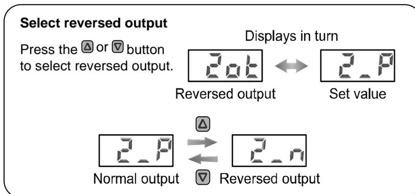
Press the **S** button to set.  $\downarrow$  Move on to setting of pressure.
