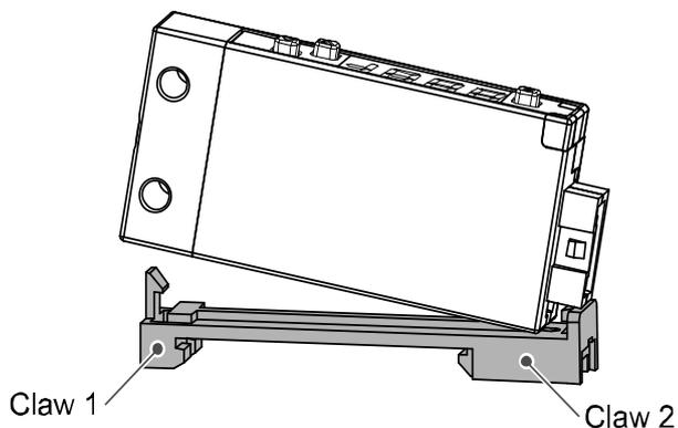
Engage the Pressure switch with claw 2 of the DIN rail adapter, then press down on to claw 1 until it clicks.
