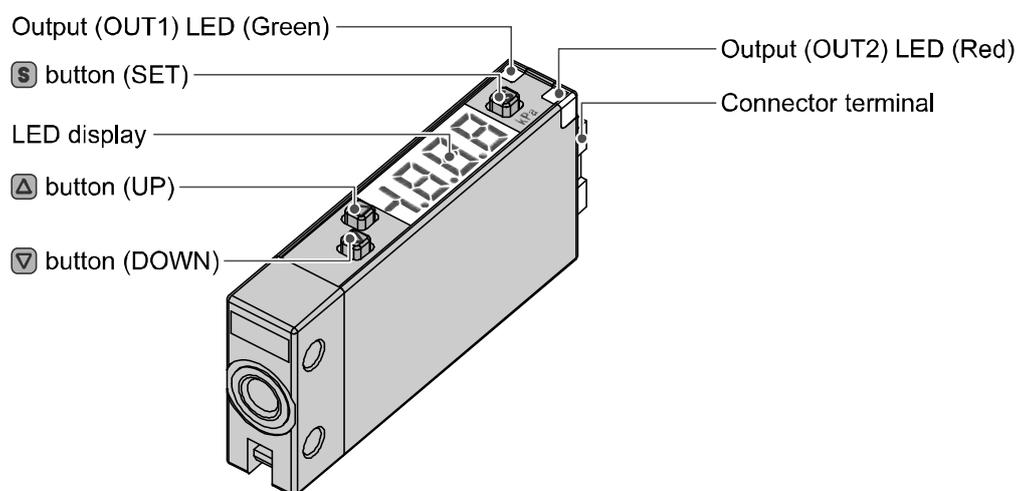
Output (OUT1) LED (Green): LED is ON when the switch output (OUT1) is ON.
