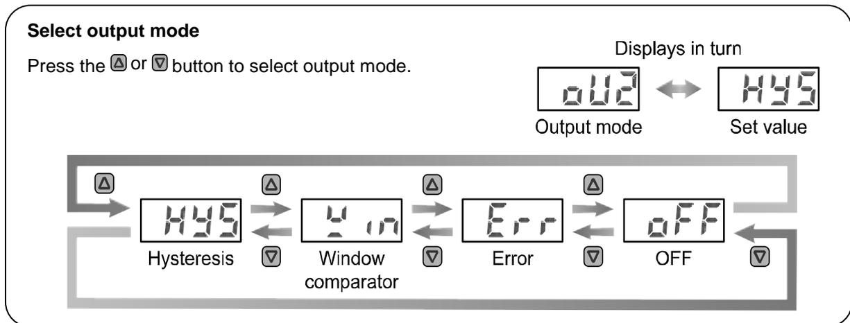
Press the **S** button to set.  $\downarrow$  Move on to setting of reversed output.
