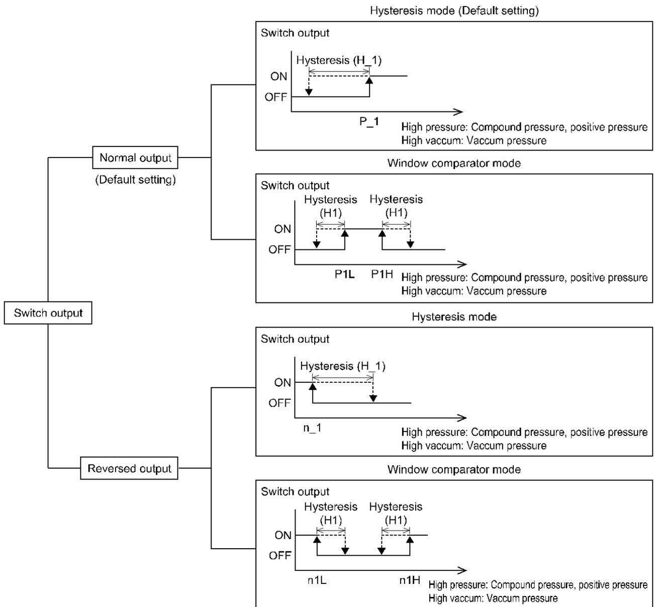
If the set point when the switch output is changed is outside the set pressure range due to switching between normal and reversed output, the hysteresis will automatically be compensated.
