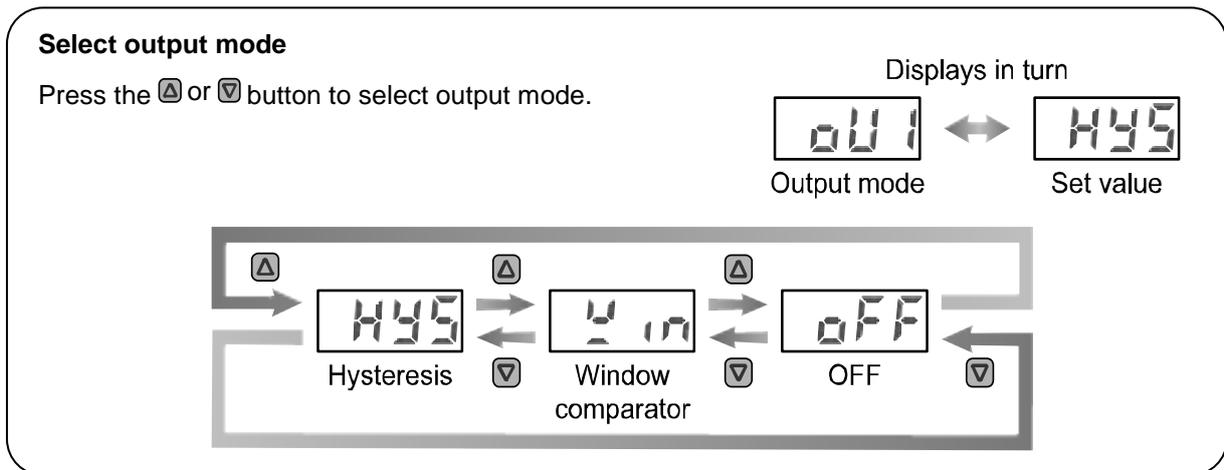
Press the  $\text{S}$  button to set.  $\downarrow$  Move on to setting of reversed output.
