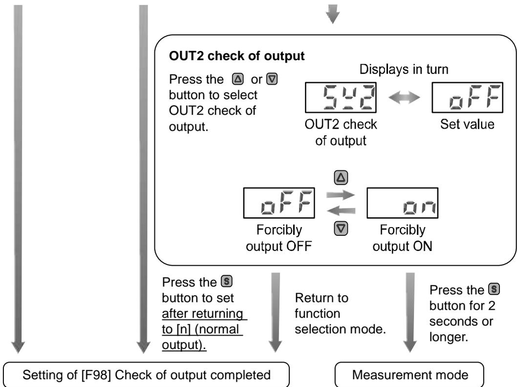
\*: If the  $\text{S}$  button is pressed for 2 seconds or longer, the mode is returned to measurement mode regardless of the current mode.
