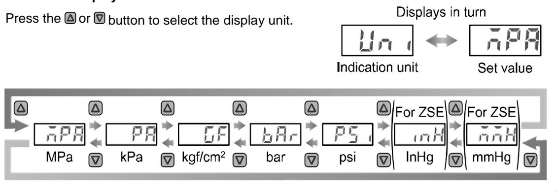
Press the  $\text{S}$  button to set.  $\downarrow$  Return to function selection mode.
