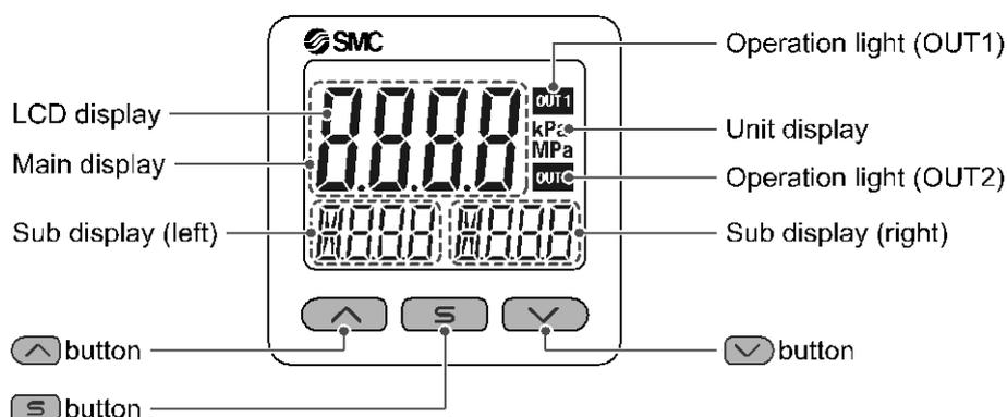
**Operation light:** Displays the switch operating condition.
