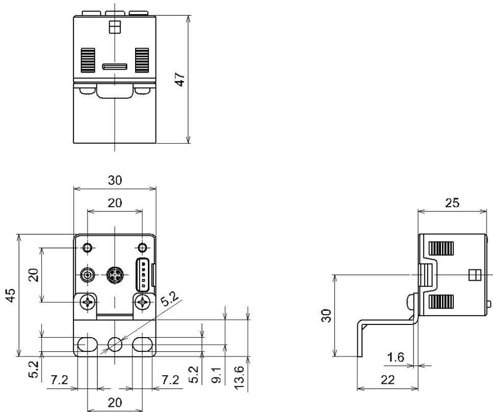
○Mounting dimensions of panel mount adapter
