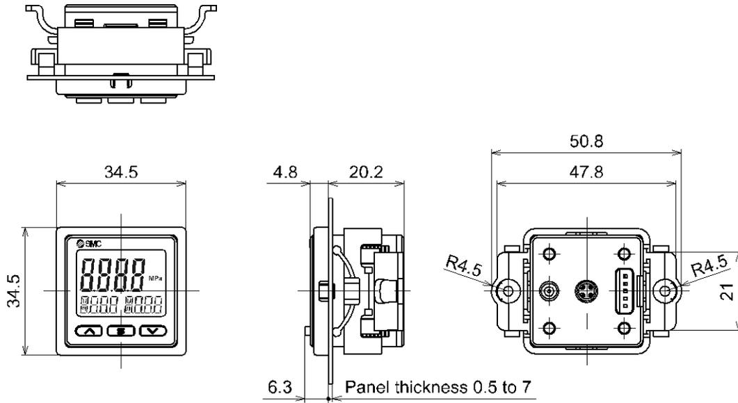
○Mounting dimension of panel mount adapter + Front protective cover
