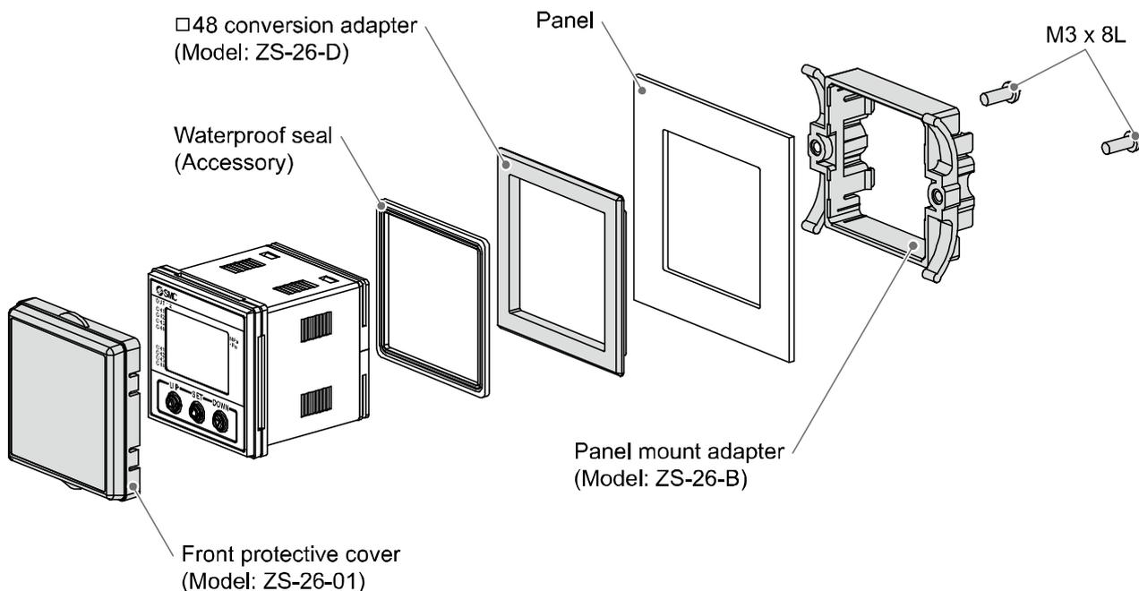
\*: The panel mount adapter can be rotated by 90 degrees for mounting.
