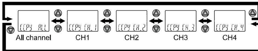
Press the SET button to start copying. When copying is finished, the mode returns to channel to channel copy function setting.
