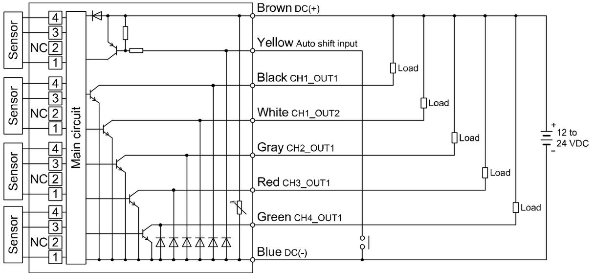
**PSE201A-(M)**: PNP open collector 5 outputs + Auto-shift 1 input
