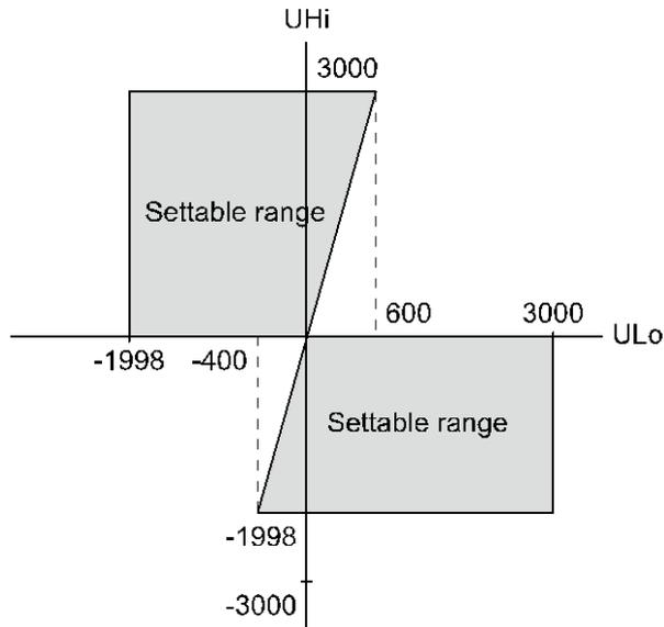
\*: When pressure range, minimum unit/lower limit/upper limit of additional range is changed, setting below will be initialized and cleared. These items must be set again.
