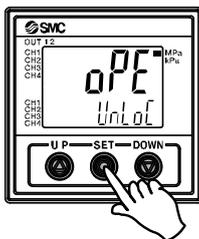
Press the UP and DOWN buttons simultaneously for 5 second or longer.
