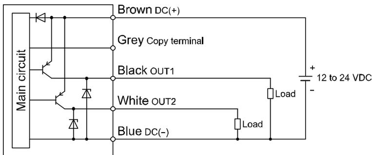
NPN (2 outputs) + analogue voltage output setting
