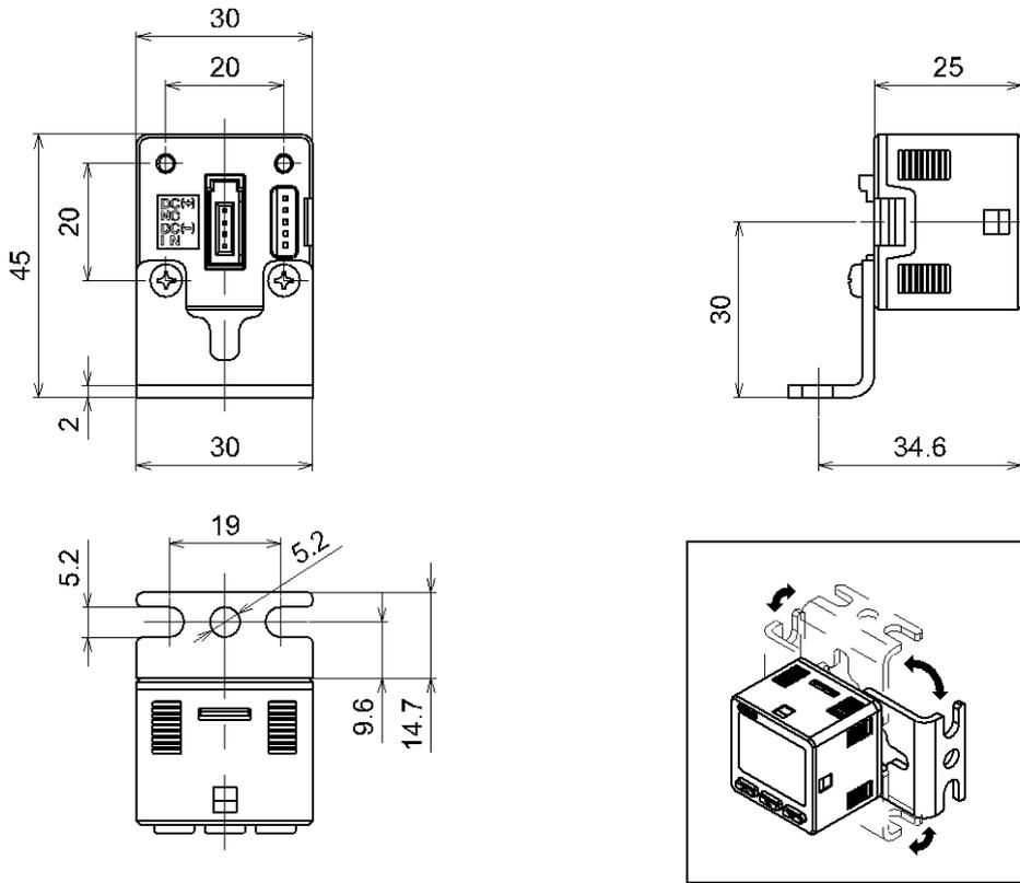
\*Bracket can be mounted on 4 sides.
