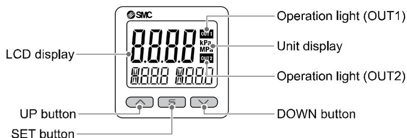
Operation light: Displays the switch operating condition.
