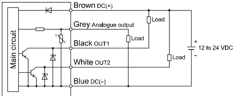
PNP (2 outputs) + analogue voltage output setting
