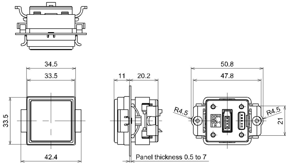
○Lead wire with connector (Part No: ZS-46-5L)
