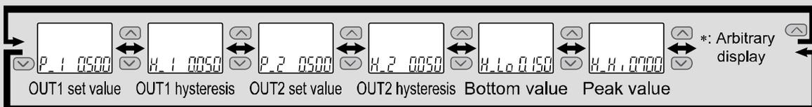
\*: One arbitrary display mode can be added to the sub display by setting the [F10] sub display setting.
