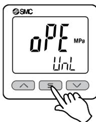
Press the UP and DOWN buttons simultaneously for 5 second or longer.
