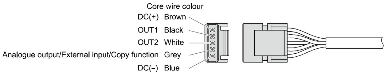
○Attaching the connector to the lead wire
