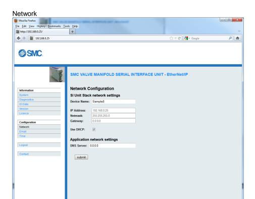
Click on Network to configure IP Address and DHCP. Device name, Netmask, Gateway, and DNS server can also be configured from this page.
