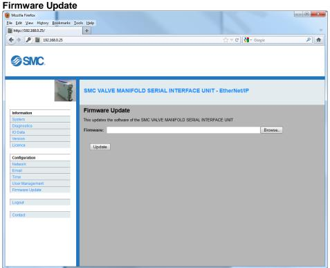
If a firmware update is required contact SMC for assistance. To download the new firmware, select the "Firmware Update" under "Configuration" tab. Browse and select the new firmware and click on Update.
