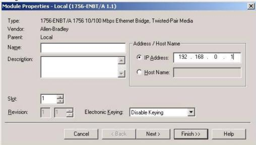
6. Right click on the EtherNet/IP scanner under I/O configuration and select New Module. We will add SMC EtherNet/IP module as Generic Ethernet Module.
