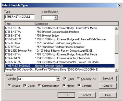
8. Name the module and enter the Comm Format, IP address and Connection Parameters.
