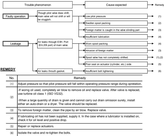
If no improvement is achieved in spite of the above countermeasure, inside of the valve may have some abnormality. In this case, stop using the valve immediately.
