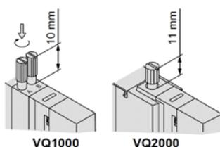
Push down on the manual override with a small flat head screwdriver or with your fingers until it stops. Turn it clockwise by 90° to lock it. Turn it counterclockwise to release it.
