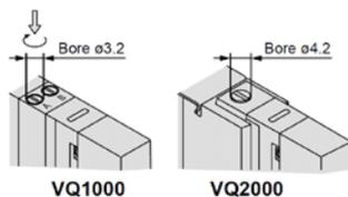
Push down on the manual override with a flat head screwdriver until it stops. Turn it clockwise by 90° to lock it. Turn it counterclockwise to release it.
