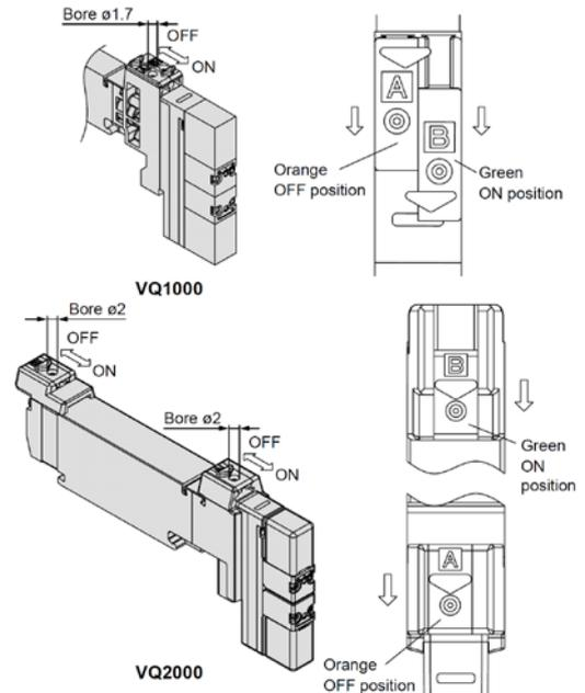
The manual override is locked by sliding it all the way to the pilot valve side (ON side) with a small flat head screwdriver or finger. Slide it to the fitting side (OFF side) to release it. In addition, it can also be used as a push type by using a screwdriver, etc., of ø1.7 or less. (ø2 or less for VQ2000).
