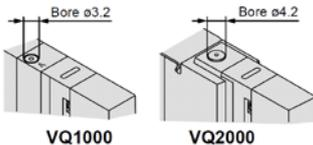
Push down on the manual override with a small screwdriver, etc. until it stops. Release the screwdriver and the manual override will return.
