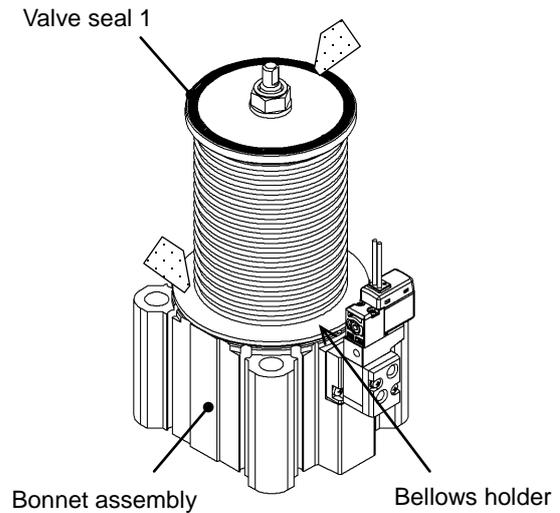
Wipe off any dust from the surfaces of the valve seal 1 and the bellows holder.
