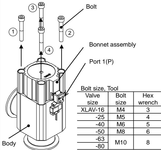
Turn ON the solenoid valve to supply air pressure of 0.4MPa (G) to the port 1(P). Loosen the bolts in numerical order to disassemble the body and the bonnet assembly. When it is difficult to remove the bonnet assembly due to adhesion of the external seal, pull the bonnet assembly straight up slowly without twisting the bonnet.
