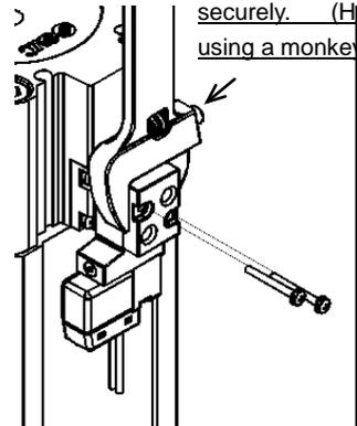
Set the parts in order of O-ring, solenoid valve, plate gasket, and plate. Tighten the screw to secure the solenoid valve.
