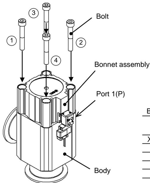
Bolt size, Tool, Tightening torque of bolt (N·m)
