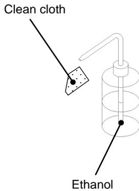
Assemble parts eliminating any dust or debris. Wipe off dust with a clean cloth soaked with ethanol. Blow parts with clean air if necessary. (Ensure there are no fibers or dust.)
