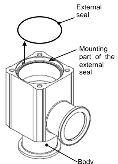
Remove the external seal from the body. (Take care not to damage the surface of the seal mounting groove.)
