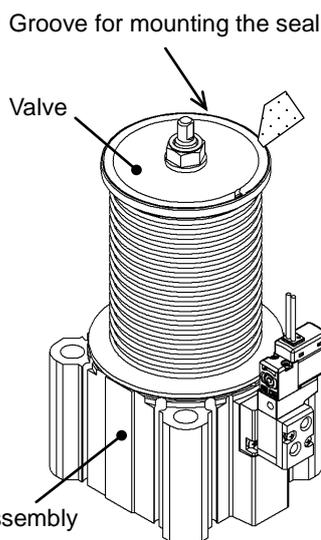
Eliminate any dust within groove for mounting the seal of the valve.
