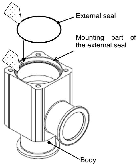
Wipe off any dust from the surface of the external seal and the mounting surface of the external seal on the body, then place the external seal in the mounting position on the body.
