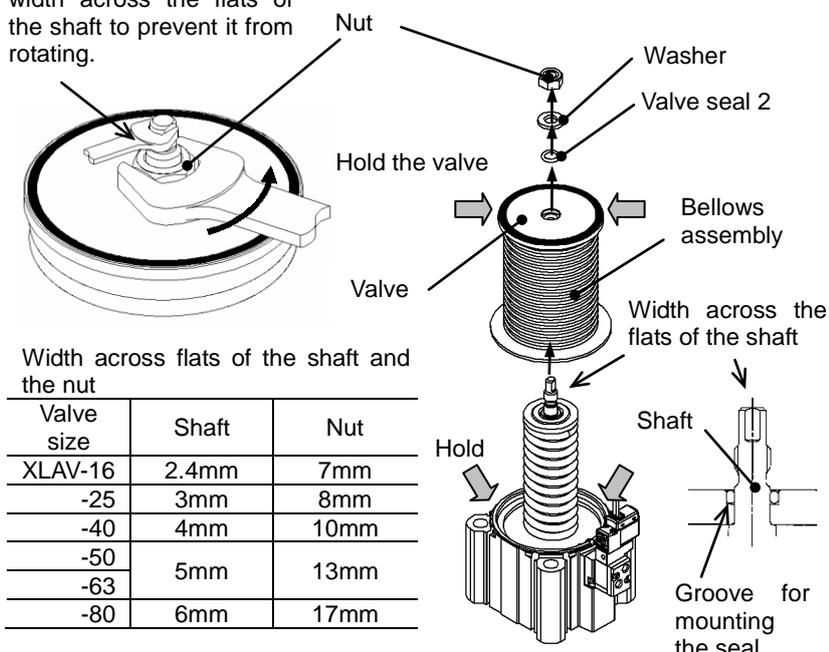
Apply a spanner to the width across the flats of the shaft of the bonnet assembly to hold the shaft, and remove the nut. Be careful not to damage the valve. Remove the washer, valve seal 2, and the bellows assembly. Be sure to hold the valve when removing the bellows assembly. Do not apply air pressure to the port 1(P) with the nut removed.
