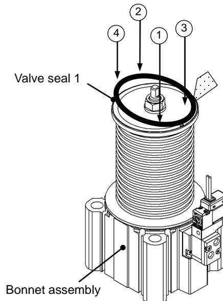
Wipe off any dust on the surface of the valve seal 1, then place the valve seal 1 in the seal mounting groove. Press the seal into the groove in numerical order (press diagonally) to fit the valve seal 1 into the groove. Do not twist the valve seal 1. Use dust-free gloves.
