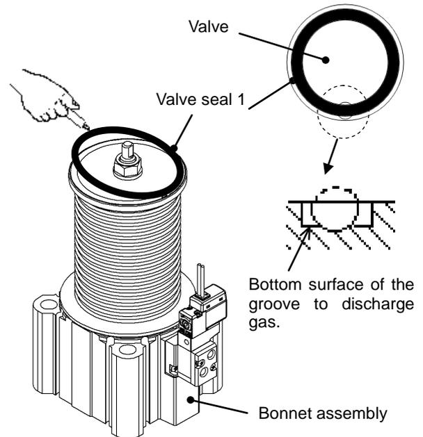
Remove the valve seal 1 from the seal mounting groove. Use a tool (e.g. which has a finger that is not longer than the depth from the bottom to the top of the groove). Use caution not to scratch the mounting groove surface of the seal.
