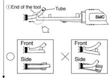
②After inserting, grasp the handle tightly and insert the end of the tubing to the stroke end.
