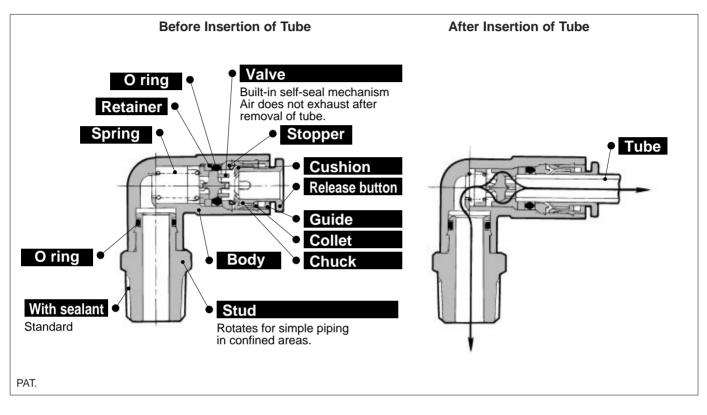
One-touch fitting (With built-in selfseal mechanism) to prevent air exhaust when removing tube.
