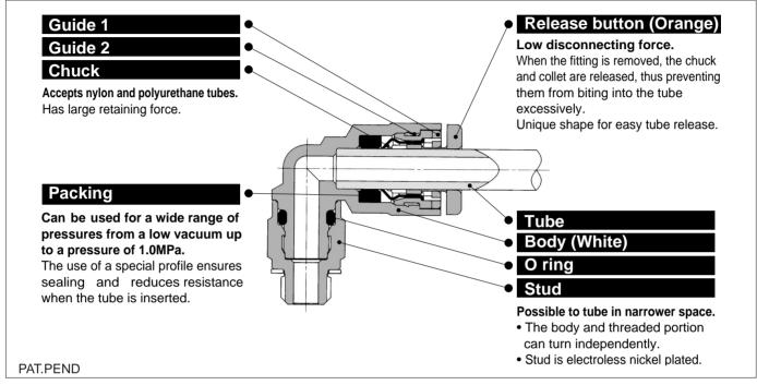
Optimum piping in less space with 20% reduction of the outside diameter
