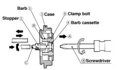
①Turn the clamp bolt ⑥ to the left with a screwdriver, loosen until the stopper ② touches the case ③, and barb cassette ④ will be pulled out in the direction ④.Then clamp portion ⑧, consisting of barb ⑤ and case ③, will be freed. Next, insert or remove the tube. ②The corresponding numbers are stamped on both the socket and plug sides for each tube connection.
