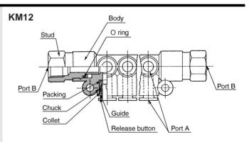
Port A: One-touch fitting Port B: NPT female thread
