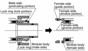
②By inserting the lock ring, the lock portion touches female side guide portion and falls into the direction shown with the arrow.
