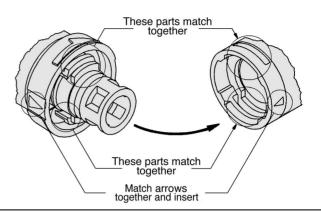
①Match arrows together and insert piping module male side into female side.
