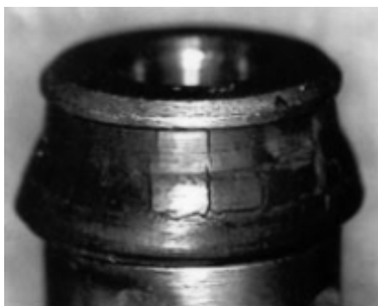
Photo 2 Cracking of check valve seal
