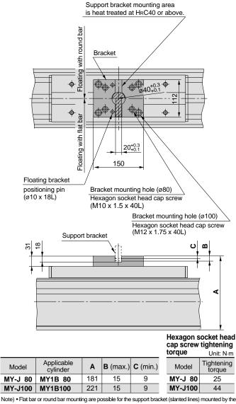
The floating bracket is packaged with (4) hexagon socket head cap screws and (2) parallel pins at
