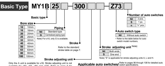
Only the A unit is available for ø16. Stroke adjusting unit is not available for ø50, ø63, ø80 and ø100. Refer to page 9 for detailed information on stroke adjusting unit specifications.
