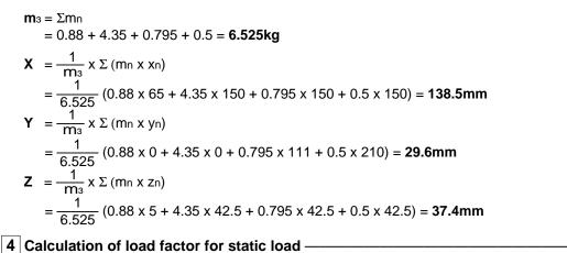
**m**<sub>3</sub>: Mass  $m_3 \max (\text{from 1 of graph MY1H/m}_3) = 50 (kg) \dots$ Load factor  $\alpha_1 = m_3 / m_3 \max = 6.525/50 = 0.13$  **M**<sub>2</sub>: Moment  $M_2 \max (\text{from 2 of graph MY1H/M}_2) = 50 (N \cdot m) \dots$   $M_2 = m_3 \times g \times Z = 6.525 \times 9.8 \times 37.4 \times 10^{-3} = 2.39 (N \cdot m)$ Load factor  $\alpha_2 = M_2/M_2 \max = 2.39/50 = 0.05$
