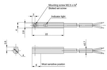
IEC529 standard IP67, watertight (JISC0920) • For a lead wire length of 3m, "L" is shown at the end of the part number. Example) D-F9NL
