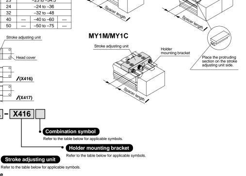
Stroke Note) Indicates the stroke prior to mounting the stroke adjusting unit.
