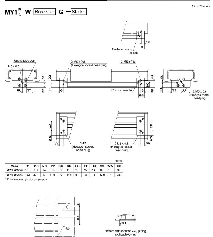
Port sizes for bottom side centralized piping (mm)
