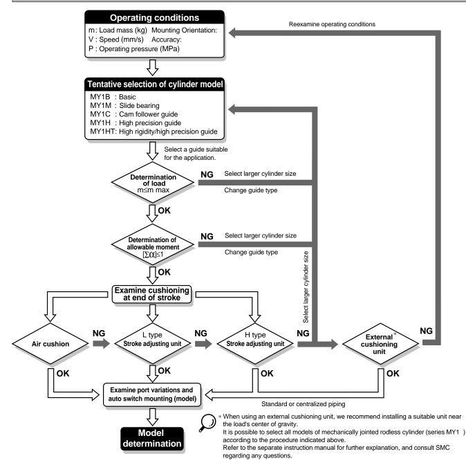
Multiple moments may be generated depending on the mounting orientation, load and position of the center of gravity.
