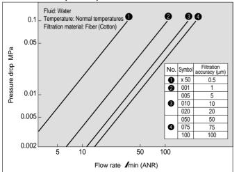
Note) The recommended flow rate is the rate for an initial pressure drop of 0.01 to 0.02 MPa.
