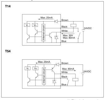
$V_L$ : Pilot valve for vacuum release  $V_S$ : Pilot valve for air supply
