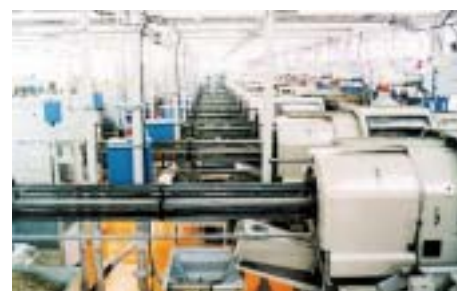
Machining line (6-axis automatic machine tools)
