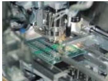
IC chip, being mounted on printed board
