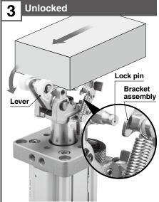
When the lock pin is unhooked from the bracket assembly, the lever becomes unlocked, which allows the workpiece to pass through.
