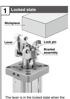
The lever is in the locked state when the lock pin is hooked on the bracket assembly.
