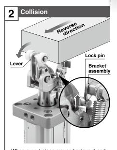
When a workpiece moves backward and collides with the lever, the lock pin unhooks from the bracket assembly as the lever is pushed backward.
