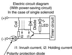
The circuit shown to the left reduces the power consumption for holding in order to save energy. Refer to the electrical power waveform as shown below.
