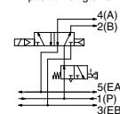
SUP stop valve spacer with residual pressure release valve
