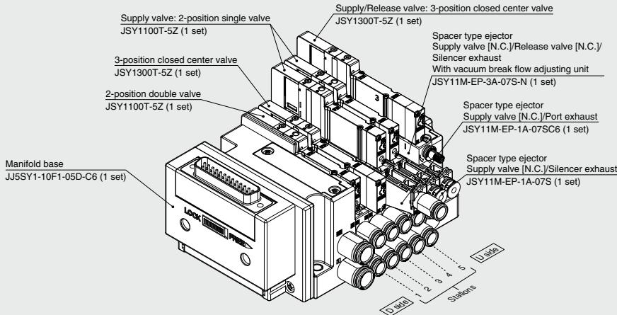
JJ5SY1-10F1-05D-C6 ..... 1 set (Type10 5stations manifold base product number/manifold block wide 9 mm limited specifications)
