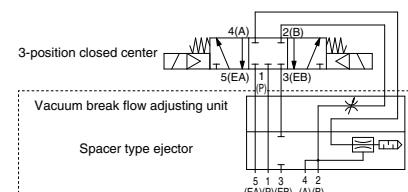
\* The valves in the above circuit diagram are examples.
