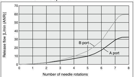
It is the vacuum release flow rate from one of the two vacuum port (A, B port). The other is turned plug.
