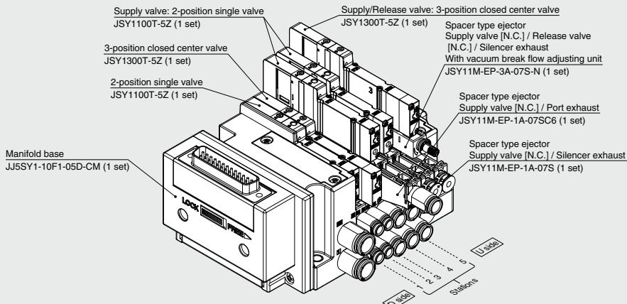
JJ5SY1-10F1-05D-CM ..... 1 set (Type10 5stations manifold base product number/manifold block width mixed specifications)
