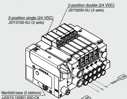
JJ5SY3-10SW2-05D-C8 ..... 1 set (Type 10 5-station manifold base part no.)
