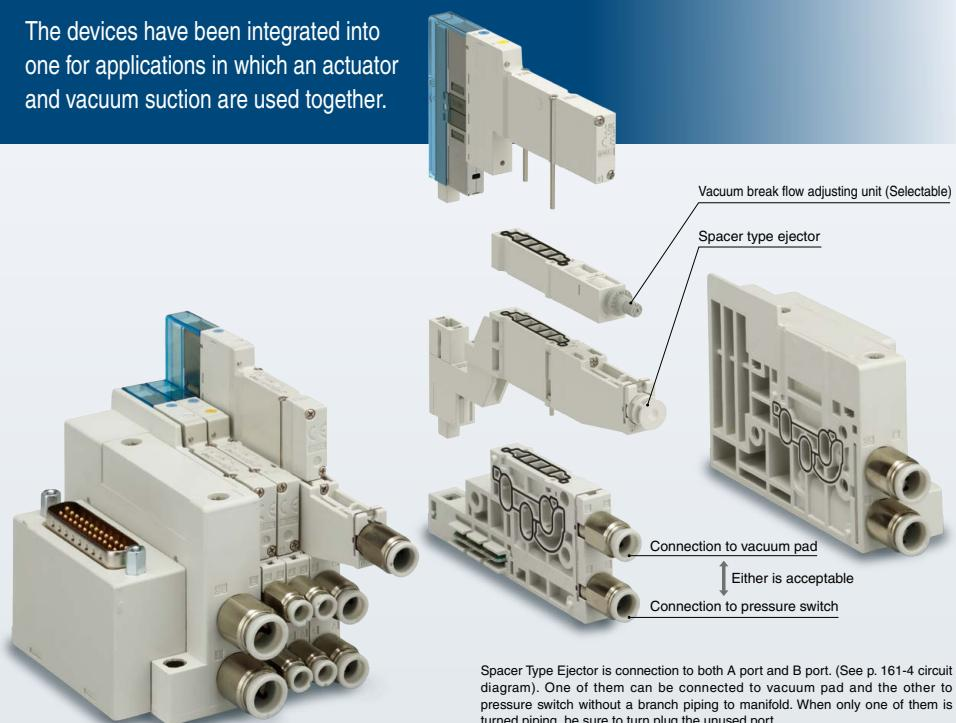
Spacer Type Ejector is connection to both A port and B port. (See p. 161-4 circuit diagram). One of them can be connected to vacuum pad and the other to pressure switch without a branch piping to manifold. When only one of them is turned piping, be sure to turn plug the unused port.
