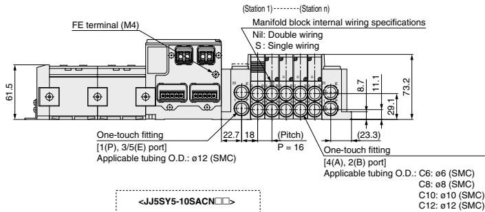
Manifold block internal wiring specifications
