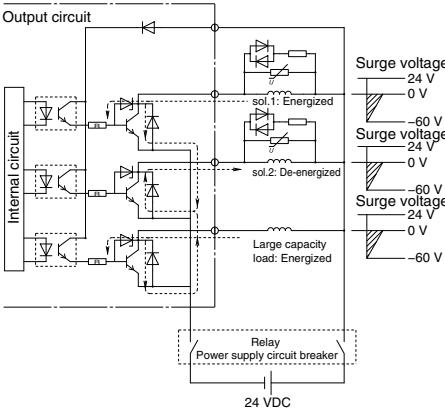
Figure 1. Surge intrusion circuit example
