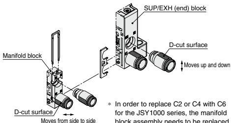
\* In order to replace C2 or C4 with C6 for the JSY1000 series, the manifold block assembly needs to be replaced. Please select the manifold block assembly on page 137.
