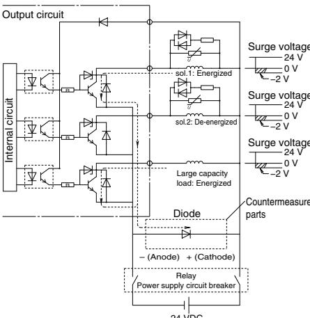
Figure 2. Surge intrusion countermeasure example
