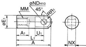
Material: Sulphur free-cutting steel
