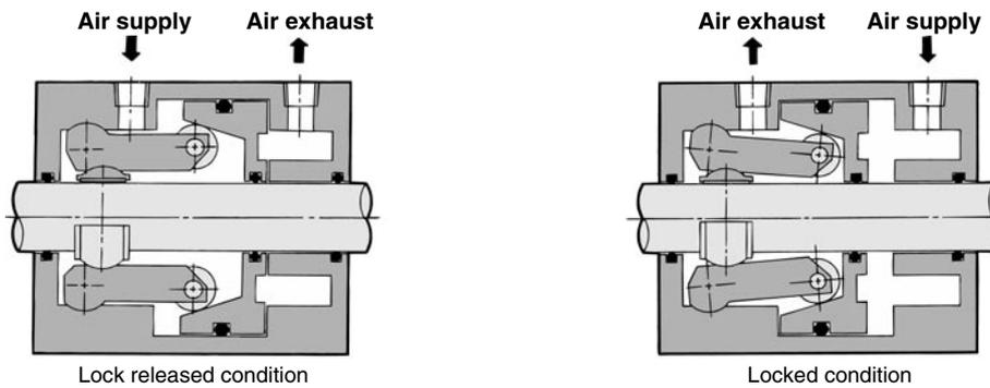
Brake piston is operated by air pressure.
