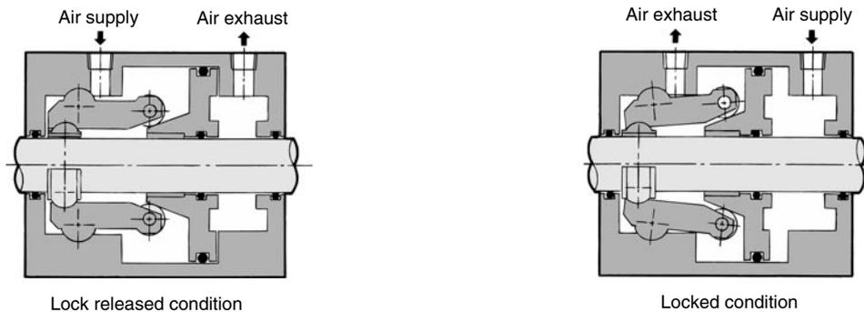
Brake piston is operated by air pressure.
