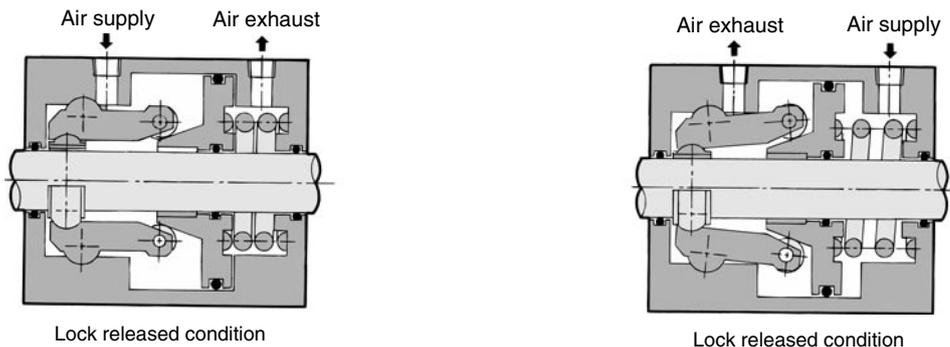
Brake piston is operated by air pressure and spring force
