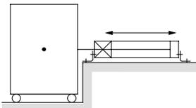
O (Load centre of gravity and cylinder axis centre are matched.)
