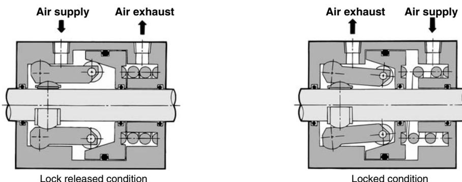
Brake piston is operated by air pressure and spring force.
