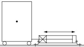
X (Load centre of gravity and cylinder axis centre are not matched.)
