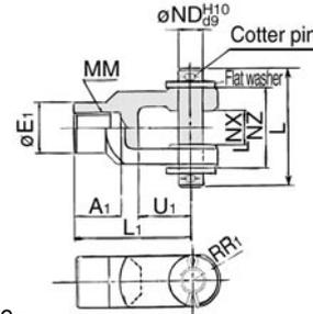
Material: Casting steel (mm)
