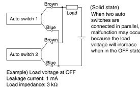
Load voltage at OFF = Leakage current x 2 pcs. x
