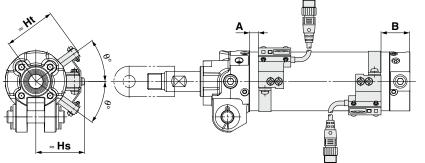
\* The above drawing is the switch band mounting example for the D-P4DWS
