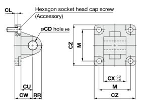
Material: Rolled steel Surface treatment: Nickel plating
