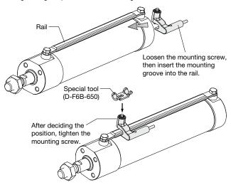
Tighten the screw within the following torque range when the auto switch mounting rail is installed during maintenance.
