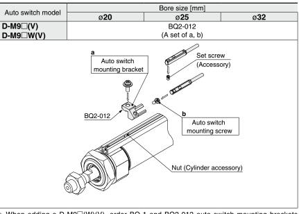
\* When adding a D-M9□(W)(V), order BQ-1 and BQ2-012 auto switch mounting brackets separately. When adding a D-F7NJ, order a BQ-1 auto switch mounting bracket separately.
