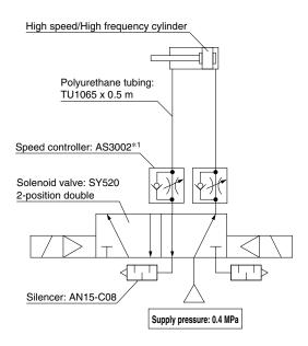
\*1 As a measure against cylinder heat generation, install the speed controller as close to the solenoid valve as possible.
