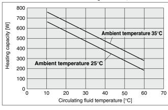
Circulating fluid: Water, Flow rate: 1 L/min, When constant fan speed mode is selected
