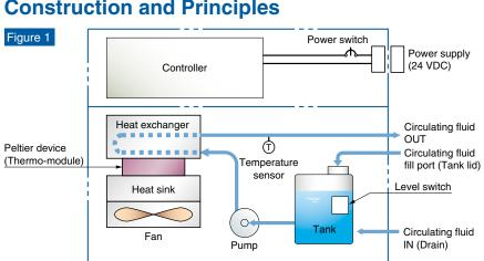
The thermo-con is constructed as shown in Figure 1. The circulating fluid outlet temperature is controlled precisely by a Peltier element (thermo module) between the heat exchanger and heat sink which is controlled by supplying DC power supply. The circulating fluid returns to the tank and is transferred by the pump which is built into the thermo-con, then it goes through the heat exchangers and temperature sensor and out from the circulating fluid outlet.
