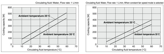
\* For the high-pressure pump (Option), the cooling capacity decreases by approx. 20 W.
