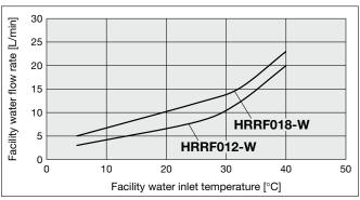
\* This is the required facility water flow rate at the circulating fluid rated flow and the cooling capacity listed in the "Cooling Capacity" specifications.
