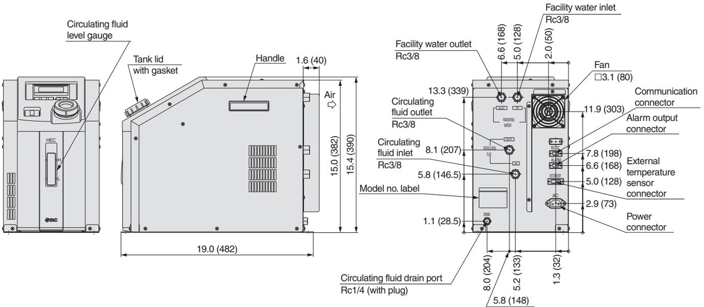
For NPT thread specification (-N), all fittings (including those at the circulating fluid drain port) are made of NPT.
