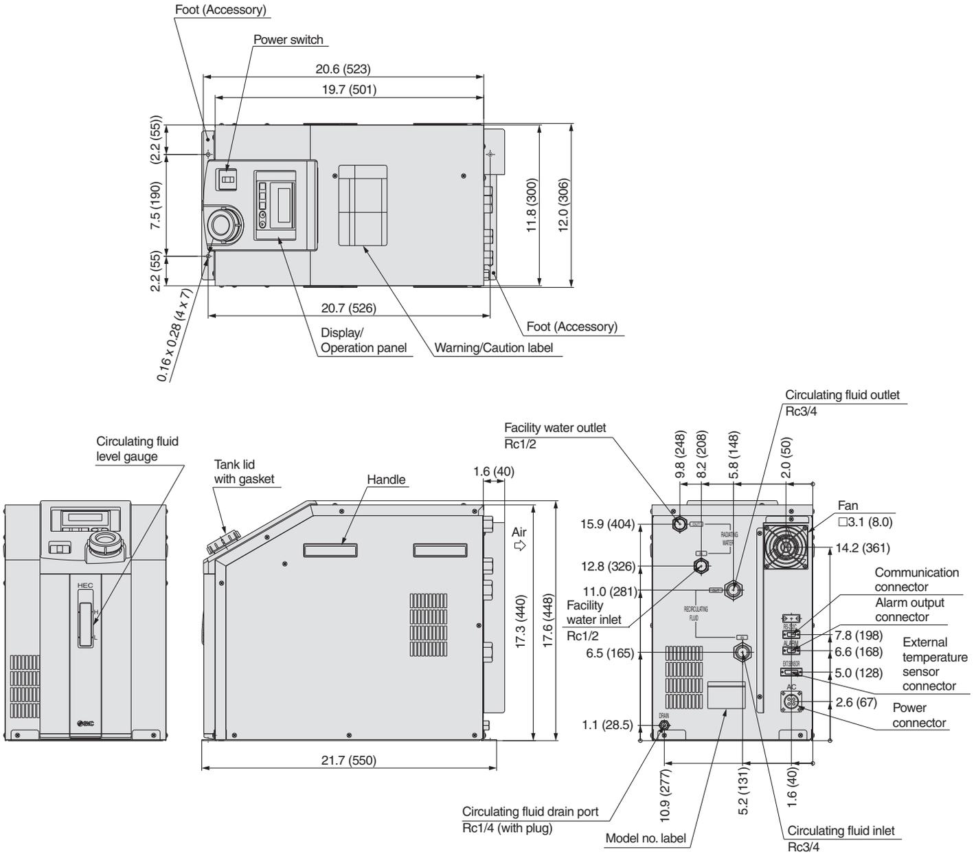
For NPT fitting specification (-N), all fittings (including those at the circulating fluid drain port) are made of NPT.
