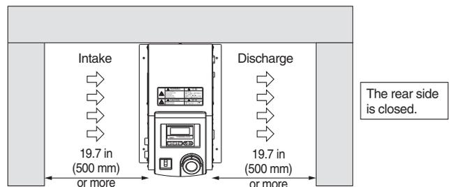
Note) The space must be 19.7 in (500 mm) or more. Be sure that the ambient temperature is within the specification range.
