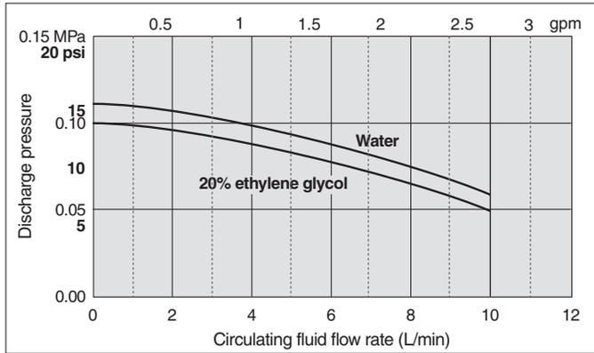
**HEC006** Since a DC pump is used, the unit is not affected by power requirements.
