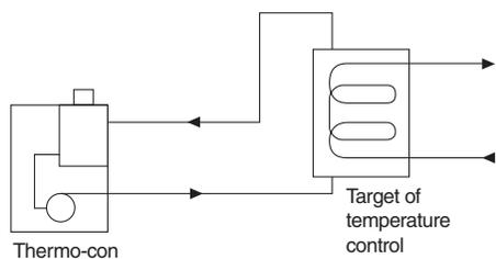
The Thermo-con is constructed as shown in Figure 1. It interposes a Peltier device (thermo-module) between the heat exchangers for the circulating fluid and facility water and controls the pulse width of supply direct current to achieve the target outlet temperature of circulating fluid precisely.
