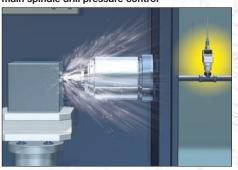
For the liquid coolant pressure control
